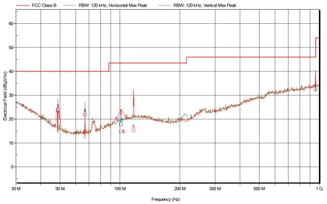
Figure 6.4.7.1: Electric field emissions Plot, 30MHz to 1GHz
