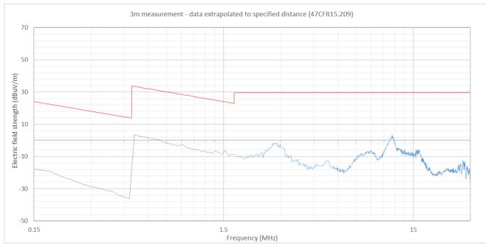
Figure 6.3.8.3: Magnetic field emissions Plot,150kHz to 30MHz Parallel orientation
