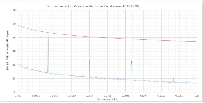
Figure 6.3.8.1: Magnetic field emissions Plot, 9kHz to 150kHz Parallel orientation
