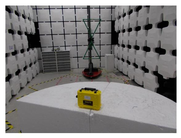
Radiated tests 30MHz to 1GHz
