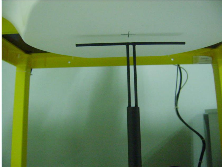
Setup Photo of Dipole Antenna
