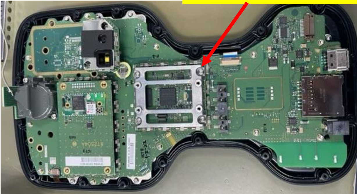
Core Module after casing removed
