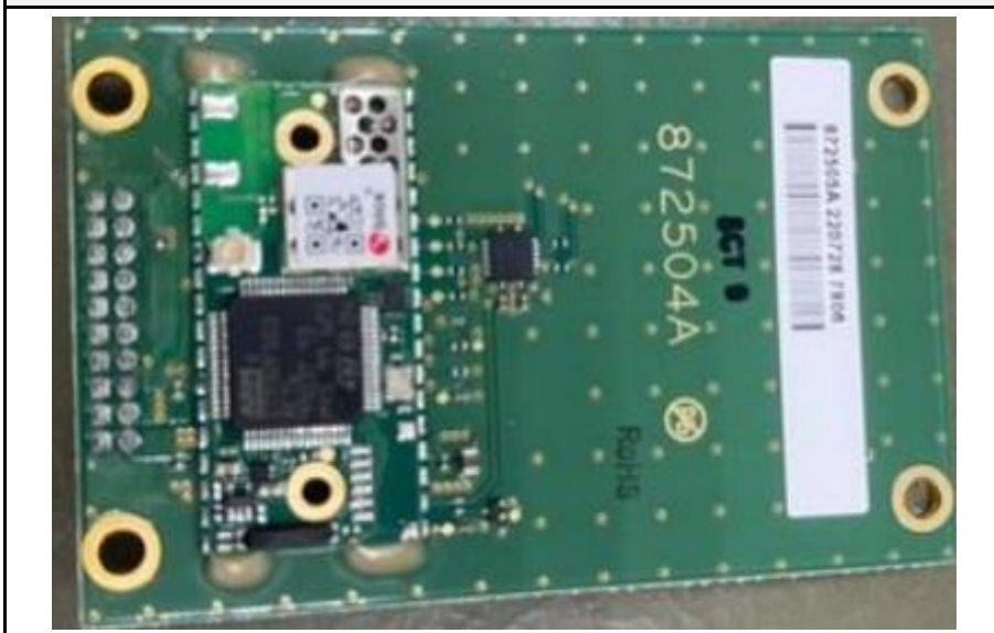
EUT PCB LONG-RANGE BLUETOOTH BOARD TOP SIDE
