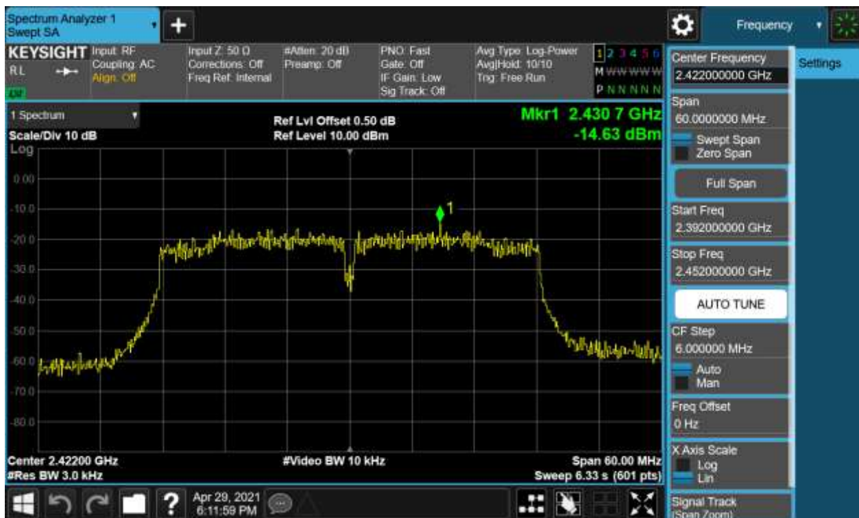
Figure 22: Power Spectral Density, 802.11n(HT40), 2422MHz
