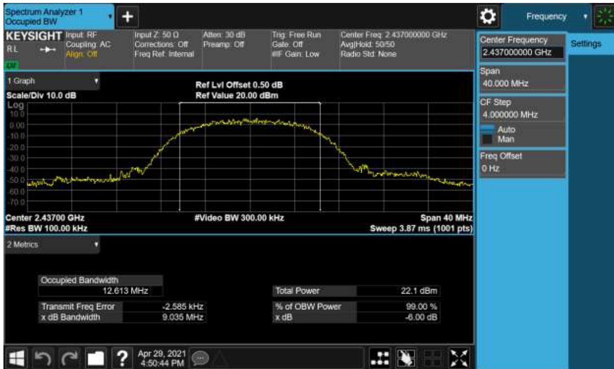
Figure 2: 6dB Bandwidth and 99% Bandwidth, 802.11b, 2437MHz
