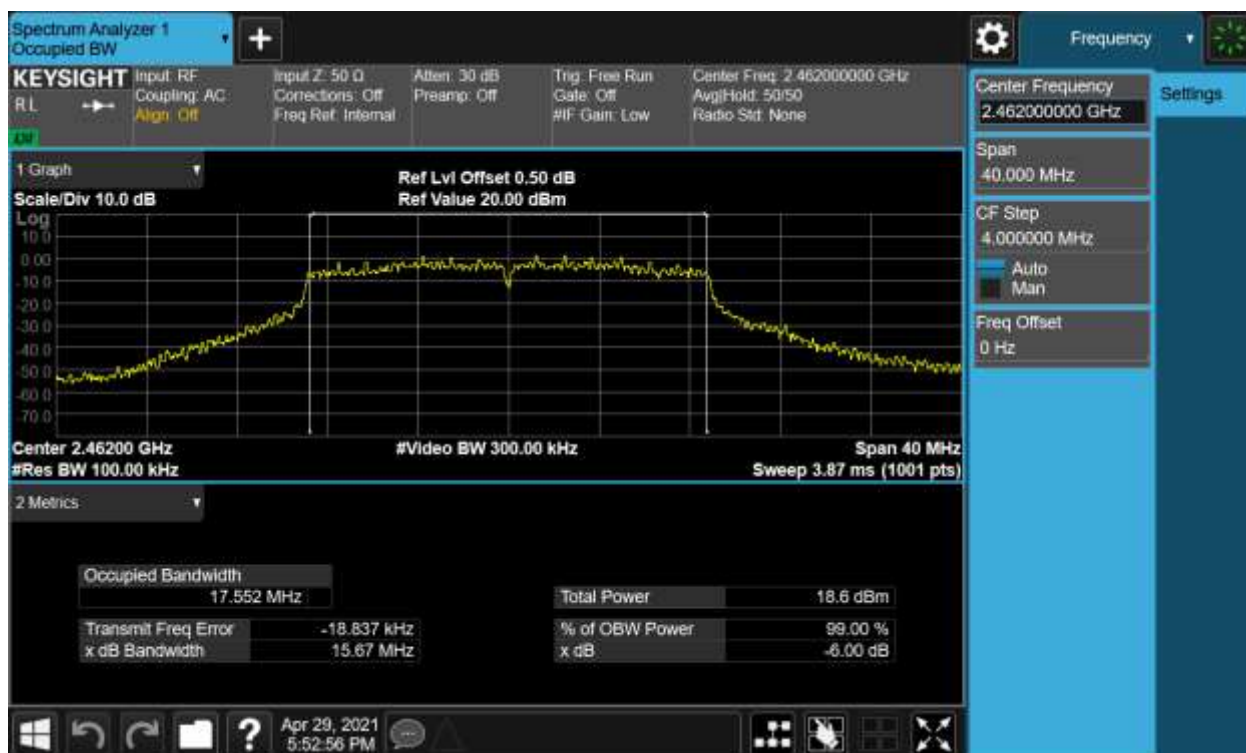
Figure 9: 6dB Bandwidth and 99% Bandwidth, 802.11n(HT20), 2462MHz
