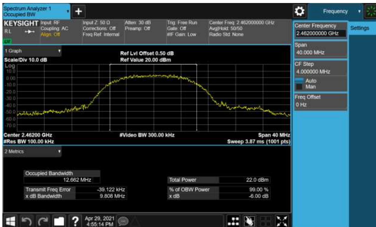
Figure 3: 6dB Bandwidth and 99% Bandwidth, 802.11b, 2462MHz
