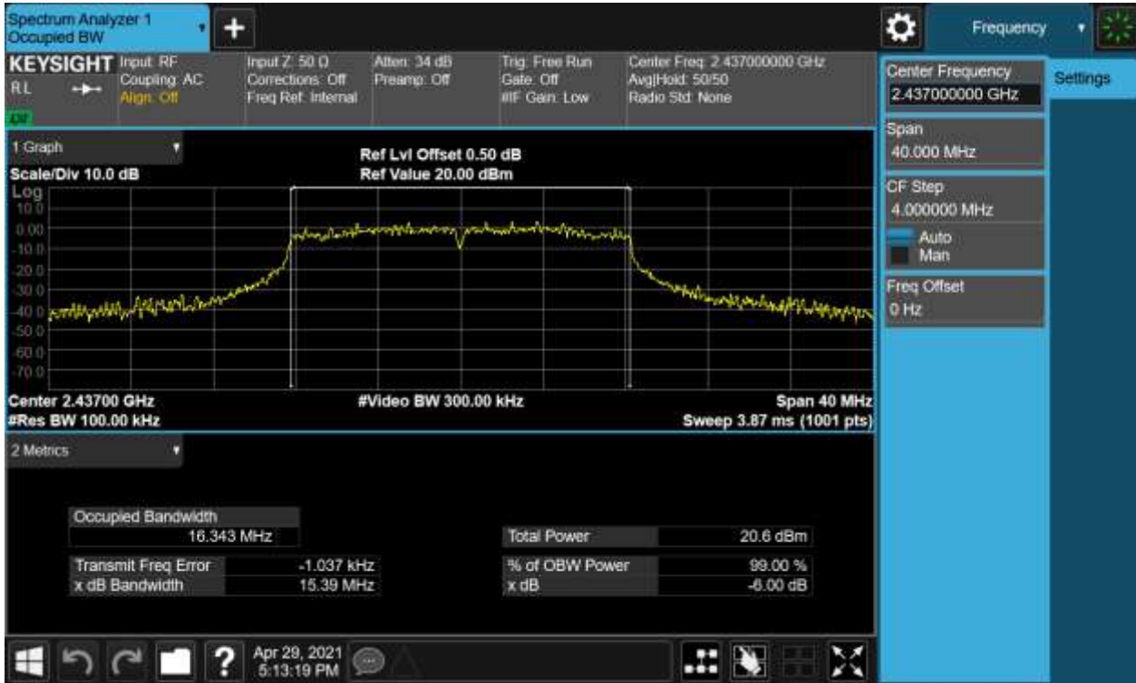
Figure 5: 6dB Bandwidth and 99% Bandwidth, 802.11g, 2437MHz
