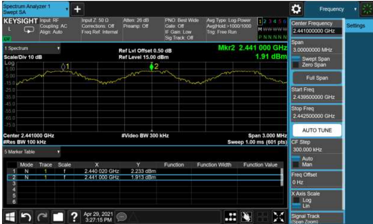
Internal Module-Hopping Frequency Separation, Hopping Mode, 8DPSK
