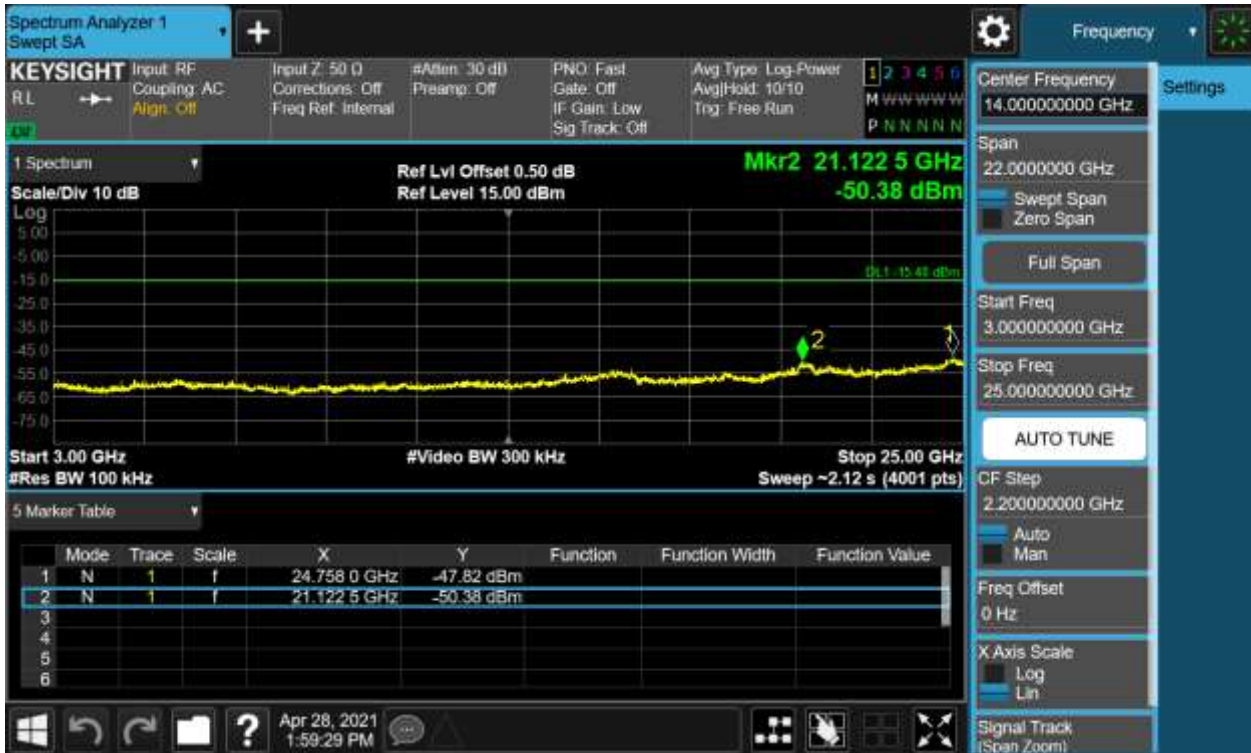
Figure 16: External Module -Conducted Spurious Emission & Authorized-band band-edge, 2402MHz, 8-DPSK Carrier Level
