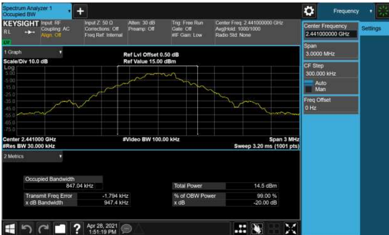
External Module-20dB Bandwidth and 99% Bandwidth, 2441MHz, GFSK
