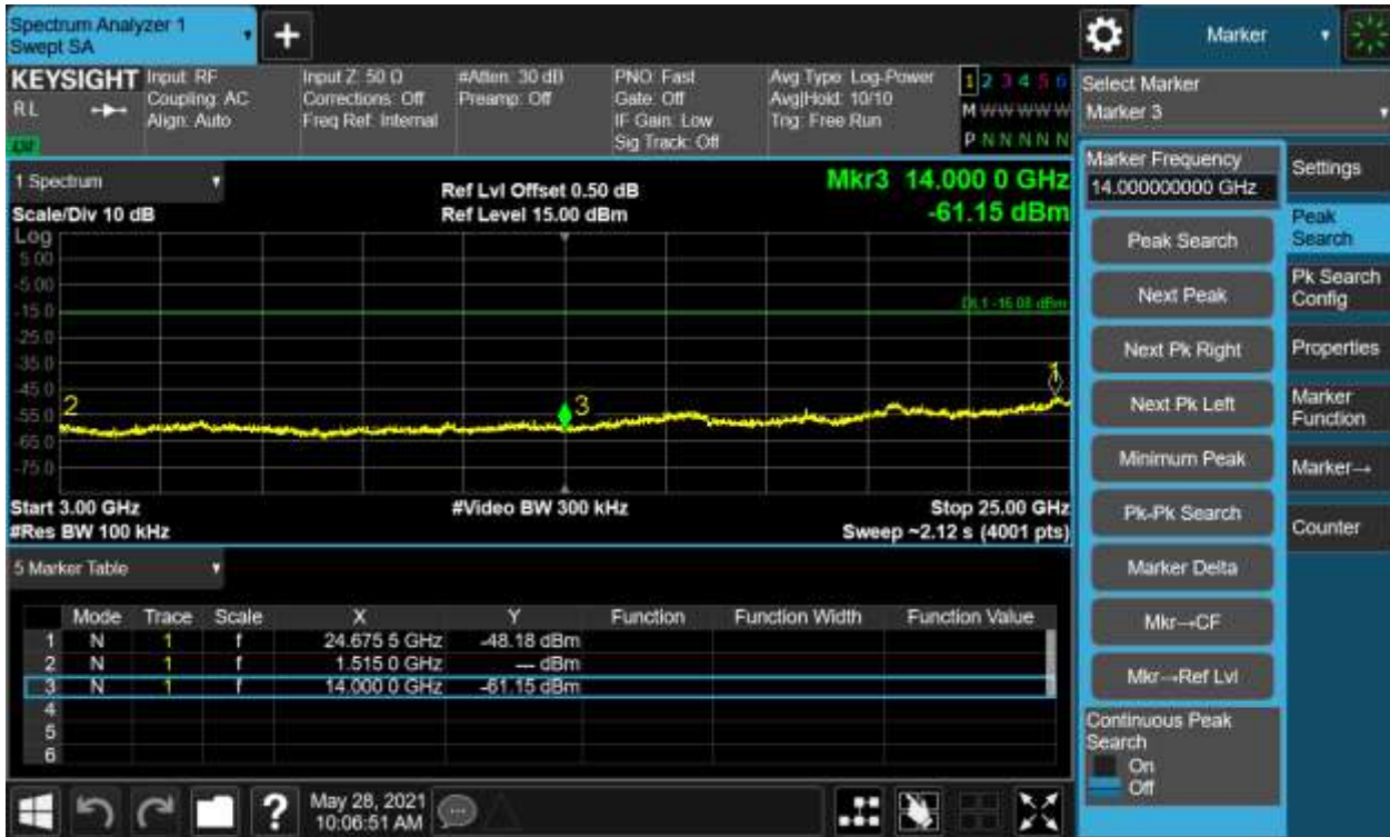
Figure 12: Internal Module-Conducted Spurious Emission & Authorized-band band-edge, Hopping Mode, 8-DPSK Carrier Level
