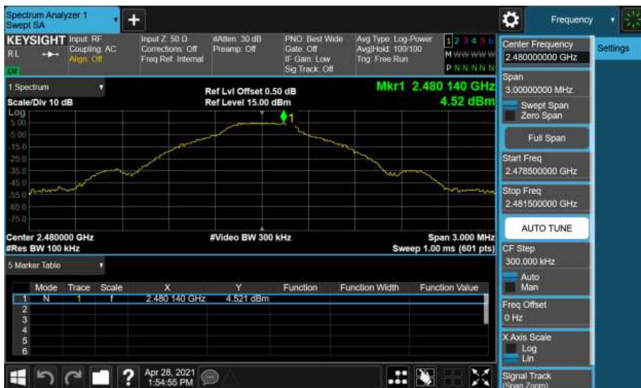
Figure 15: External Module -Conducted Spurious Emission & Authorized-band band-edge, 2480, GFSK Carrier Level
