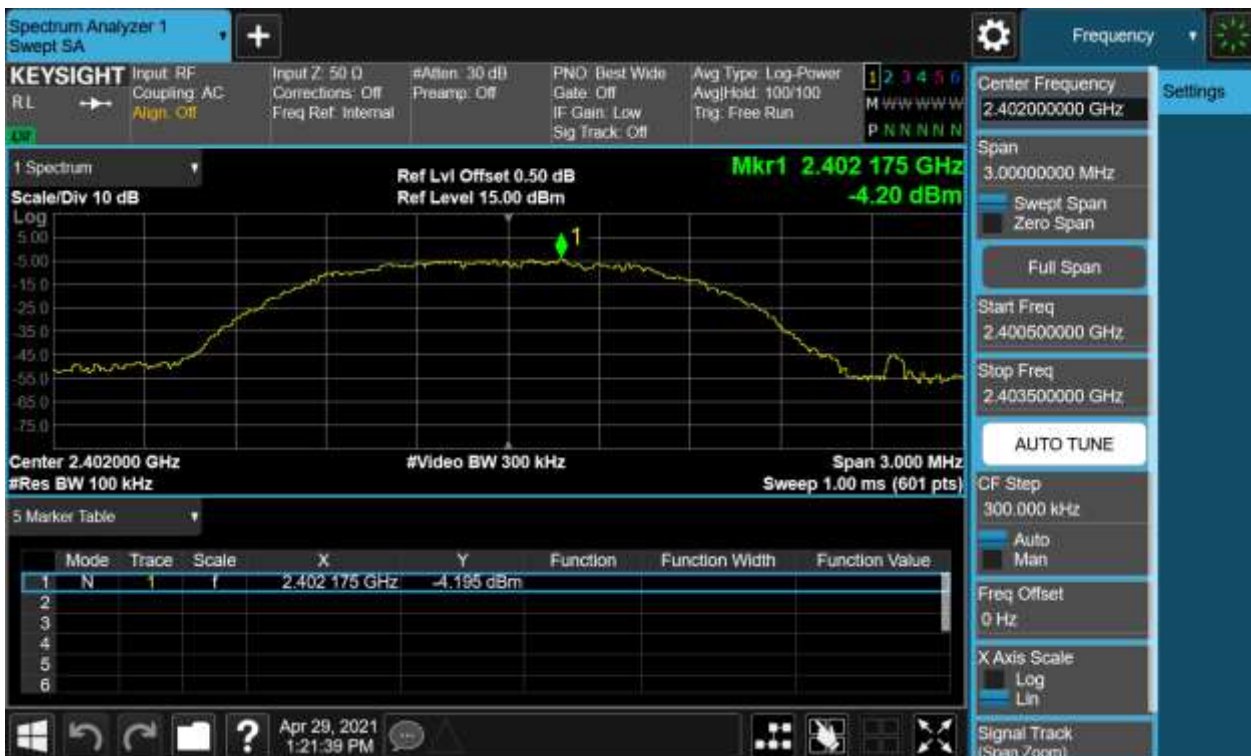
Figure 8: Internal Module-Conducted Spurious Emission & Authorized-band band-edge, 2402MHz, 8-DPSK Carrier Level
