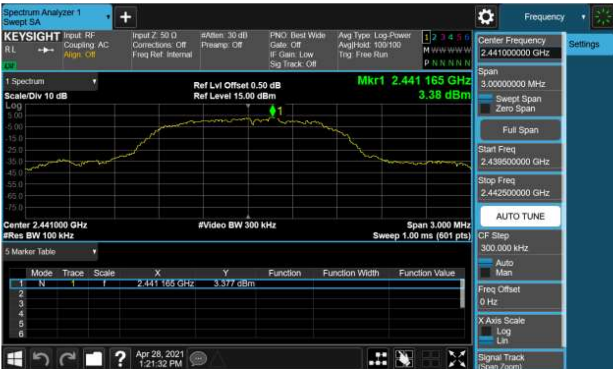
Figure 17: External Module -Conducted Spurious Emission & Authorized-band band-edge, 2441MHz, 8-DPSK Carrier Level
