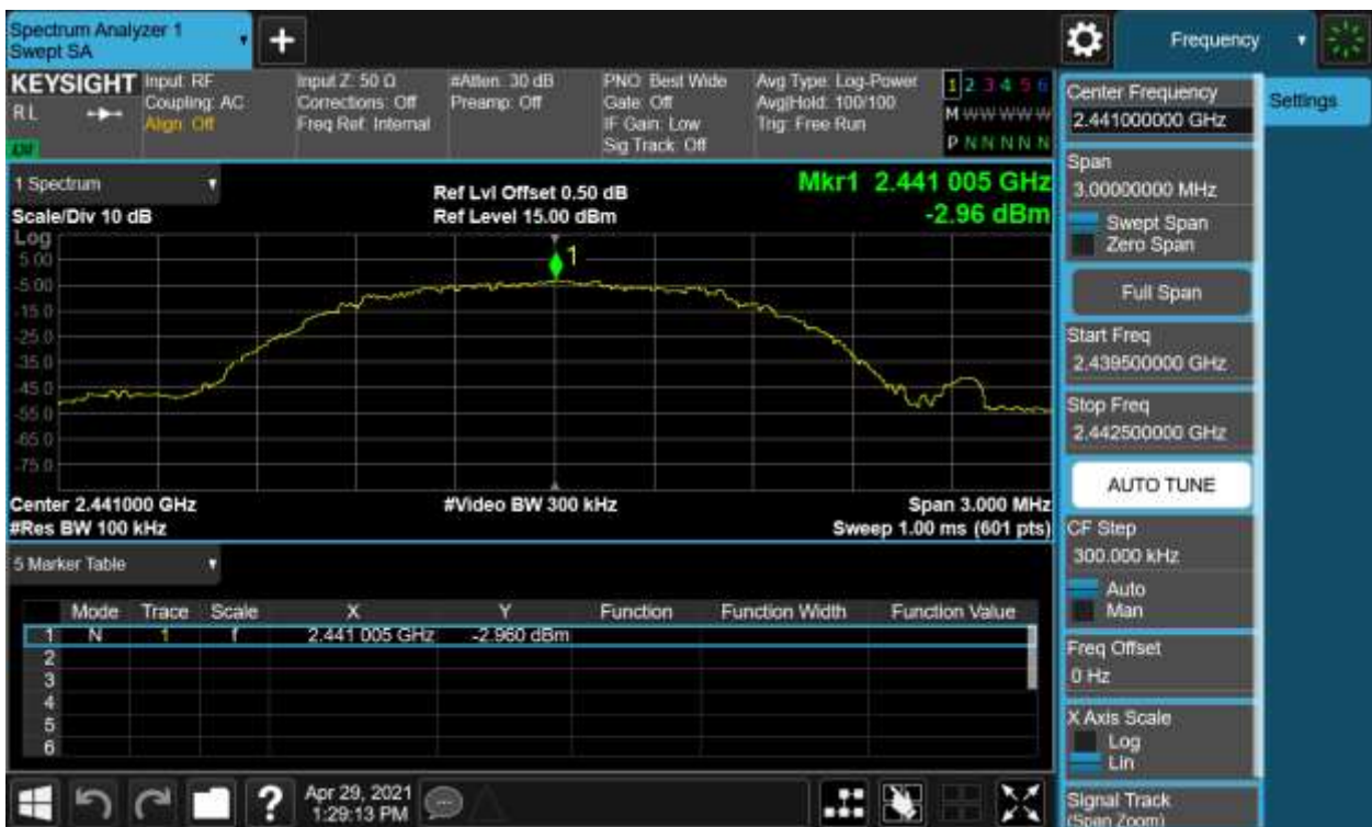
Figure 9: Internal Module-Conducted Spurious Emission & Authorized-band band-edge, 2441MHz, 8-DPSK Carrier Level
