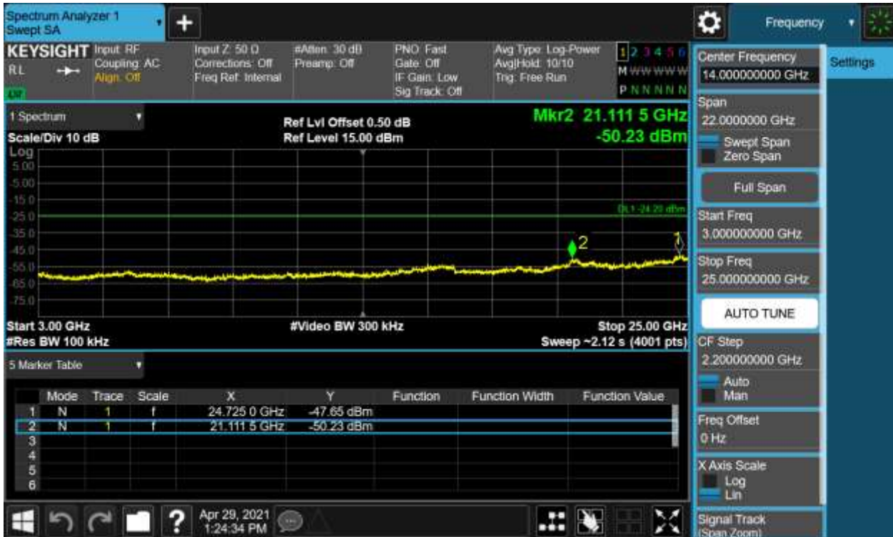
Figure 9: Internal Module-Conducted Spurious Emission & Authorized-band band-edge, 2441MHz, 8-DPSK Carrier Level
