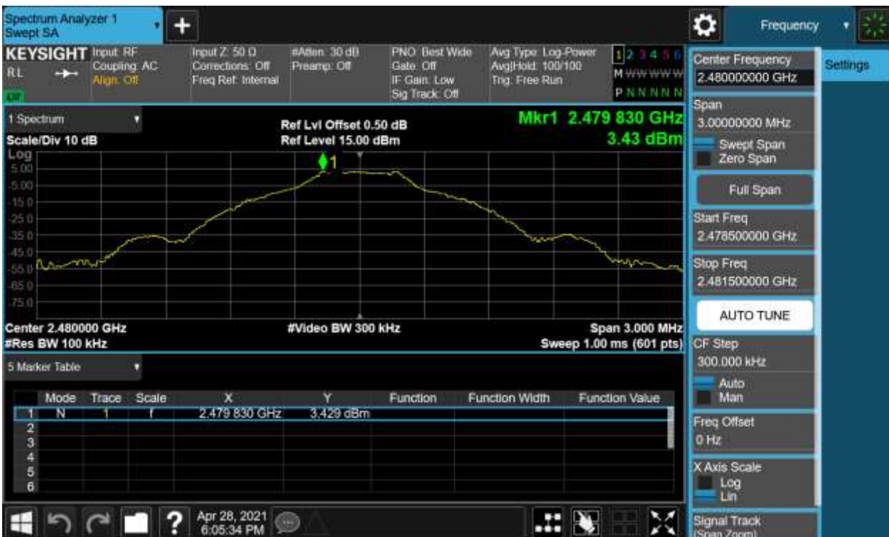
Figure 7: Internal Module-Conducted Spurious Emission & Authorized-band band-edge, 2480MHz, GFSK Carrier Level
