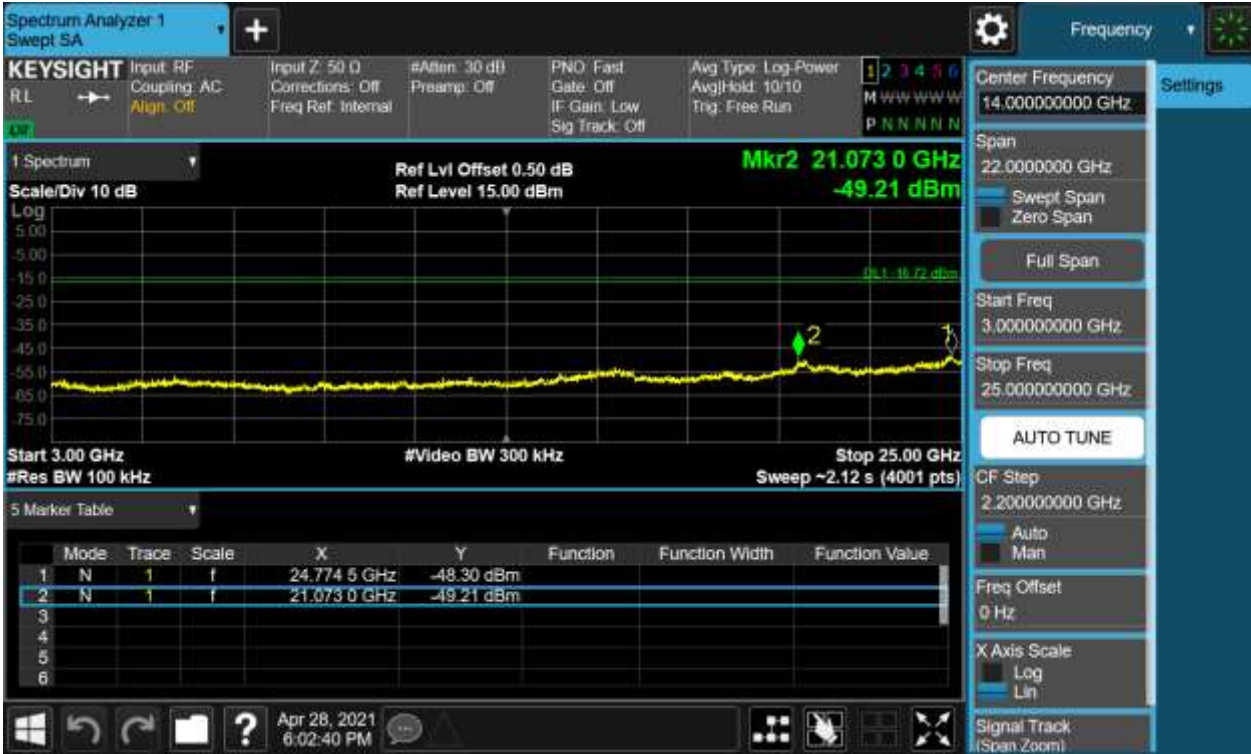
Figure 7: Internal Module-Conducted Spurious Emission & Authorized-band band-edge, 2480MHz, GFSK Carrier Level
