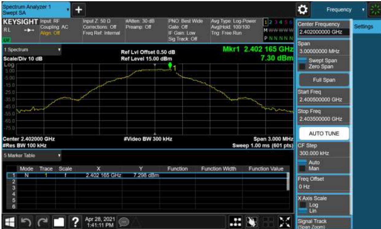
Figure 13: External Module -Conducted Spurious Emission & Authorized-band band-edge, 2402, GFSK Carrier Level
