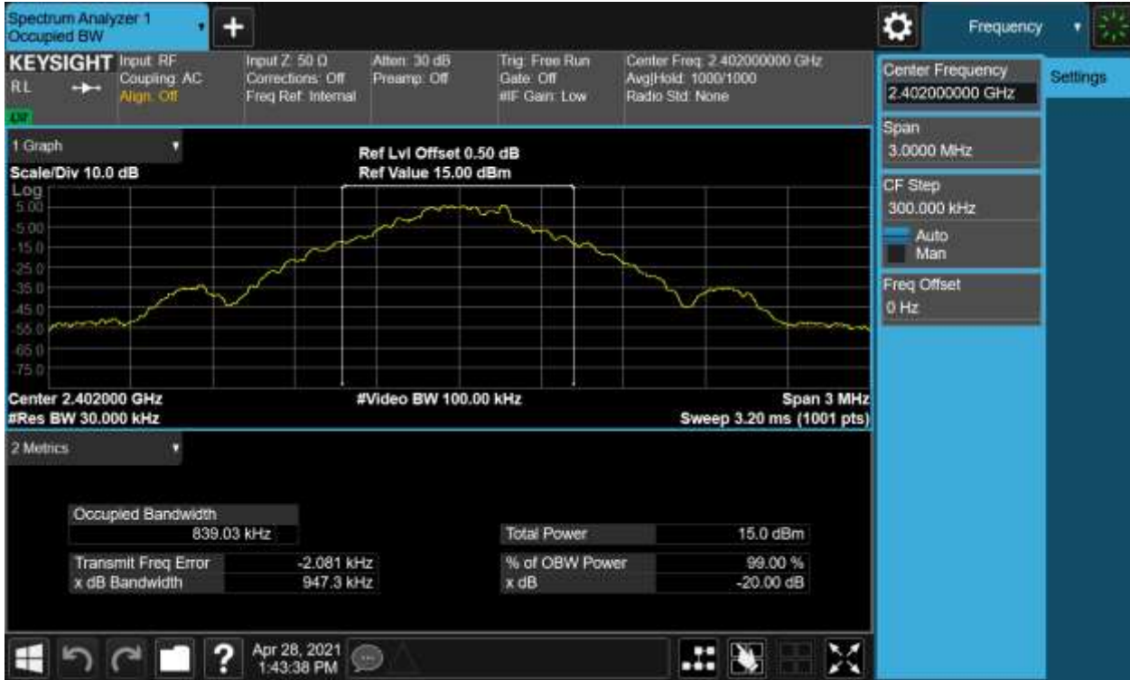
External Module-20dB Bandwidth and 99% Bandwidth, 2441MHz, GFSK
