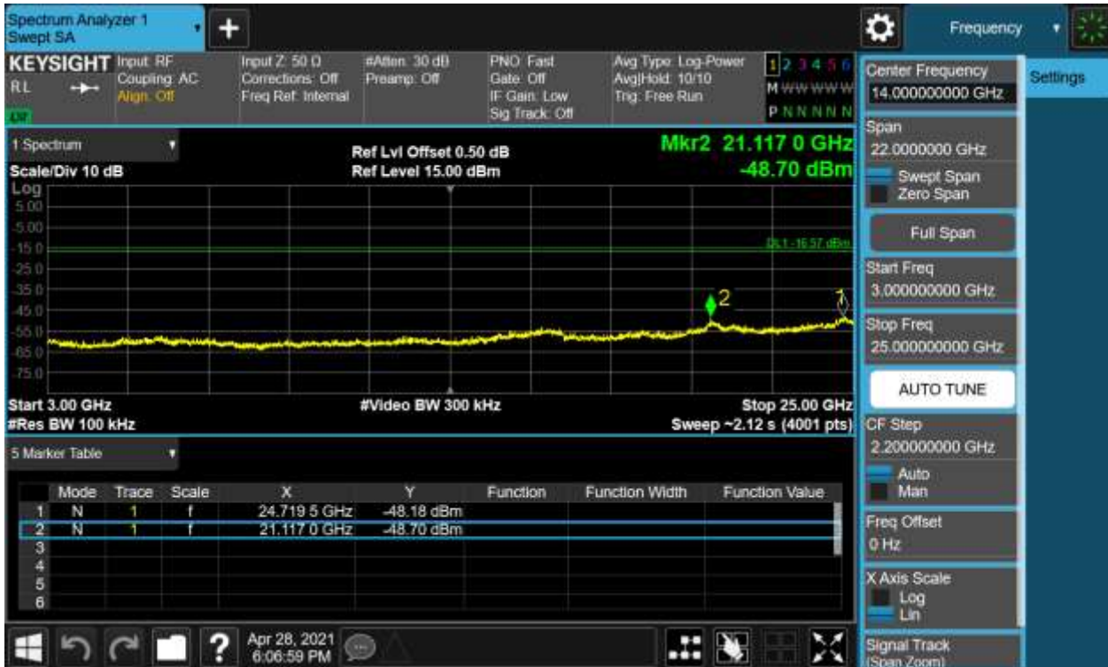
Figure 8: Internal Module-Conducted Spurious Emission & Authorized-band band-edge, 2402MHz, 8-DPSK Carrier Level
