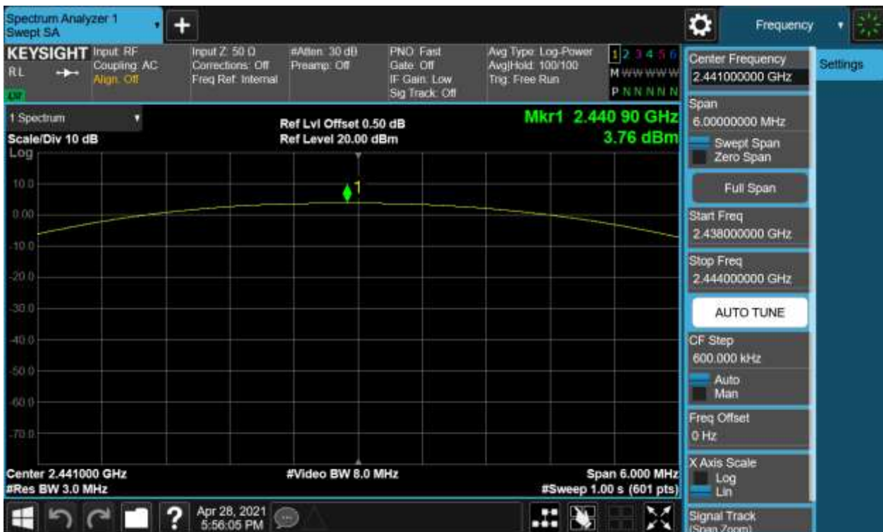
Internal Module-Maximum Conducted Output Power, 2441MHz, GFSK
