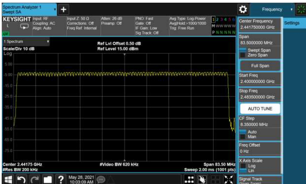
Internal Module-Number of Hopping Frequency, Hopping Mode, 8-DPSK
