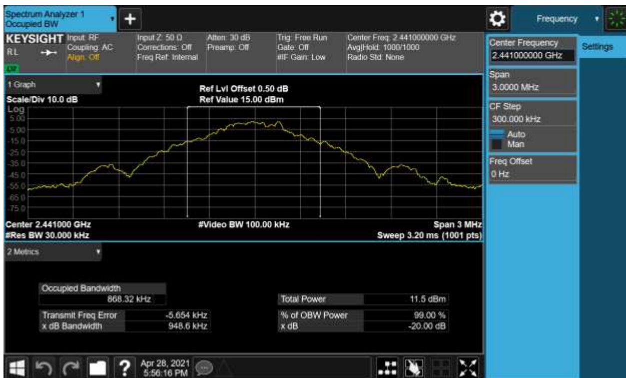
Internal Module-20dB Bandwidth and 99% Bandwidth, 2441MHz, GFSK
