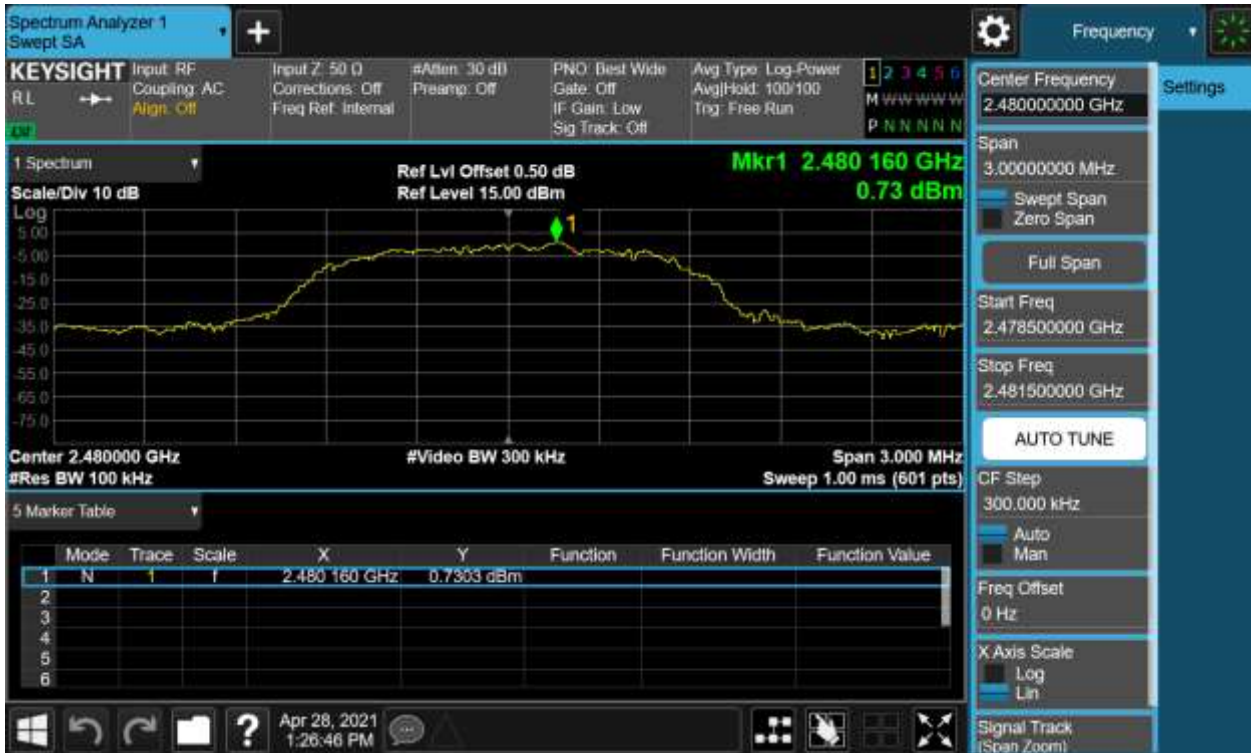
Figure 18: External Module -Conducted Spurious Emission & Authorized-band band-edge, 2480MHz, 8-DPSK Carrier Level
