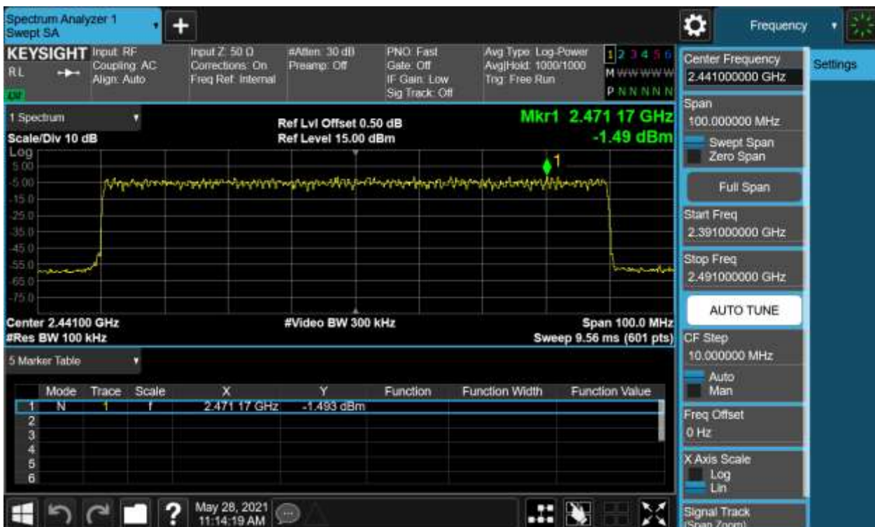
Figure 12: Internal Module-Conducted Spurious Emission & Authorized-band band-edge, Hopping Mode, 8-DPSK Carrier Level
