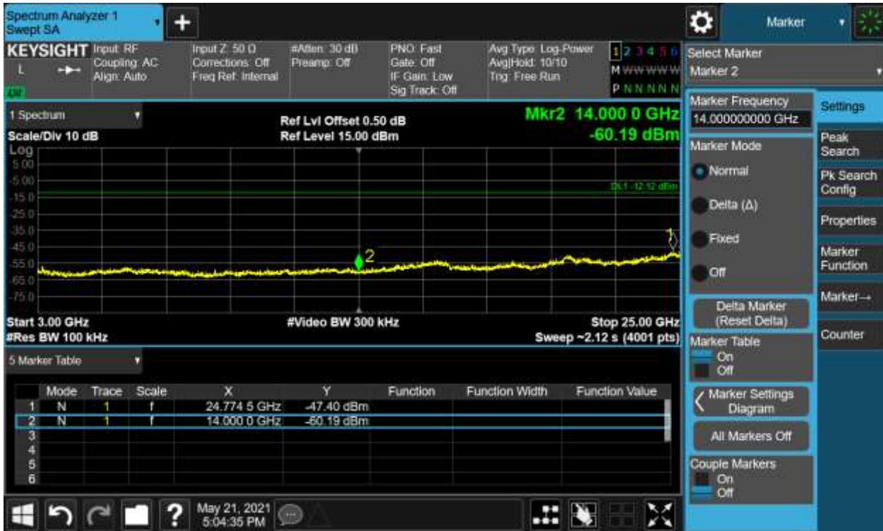
Figure 19: External Module -Conducted Spurious Emission & Authorized-band band-edge, Hopping mode, 8-DPSK Carrier Level
