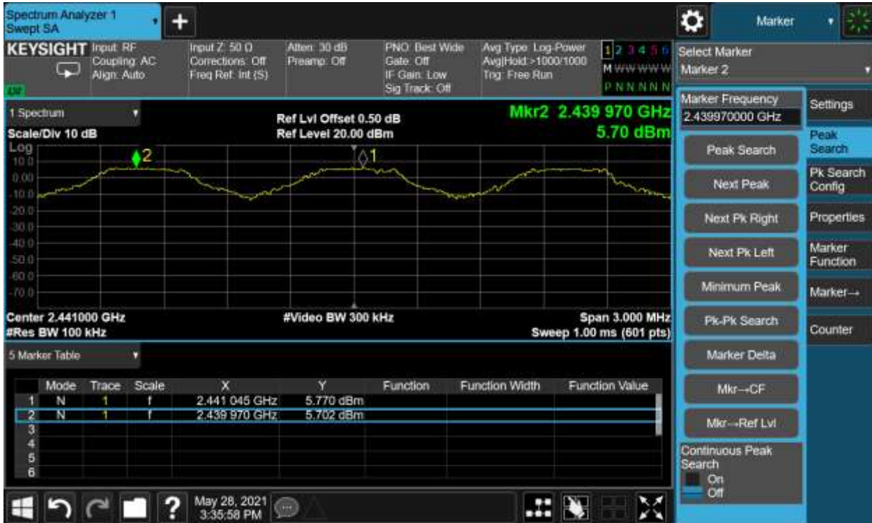
External Module-Hopping Frequency Separation, Hopping Mode, 8DPSK
