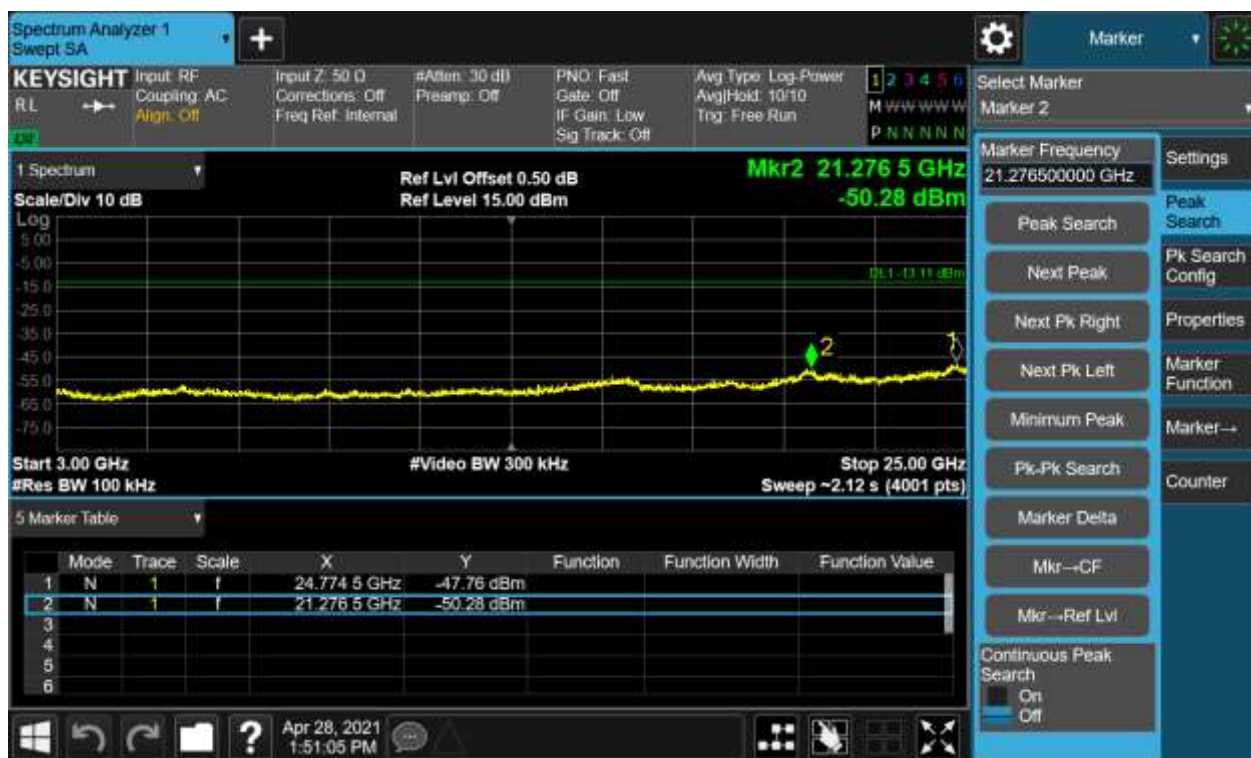
Figure 15: External Module -Conducted Spurious Emission & Authorized-band band-edge, 2480, GFSK Carrier Level
