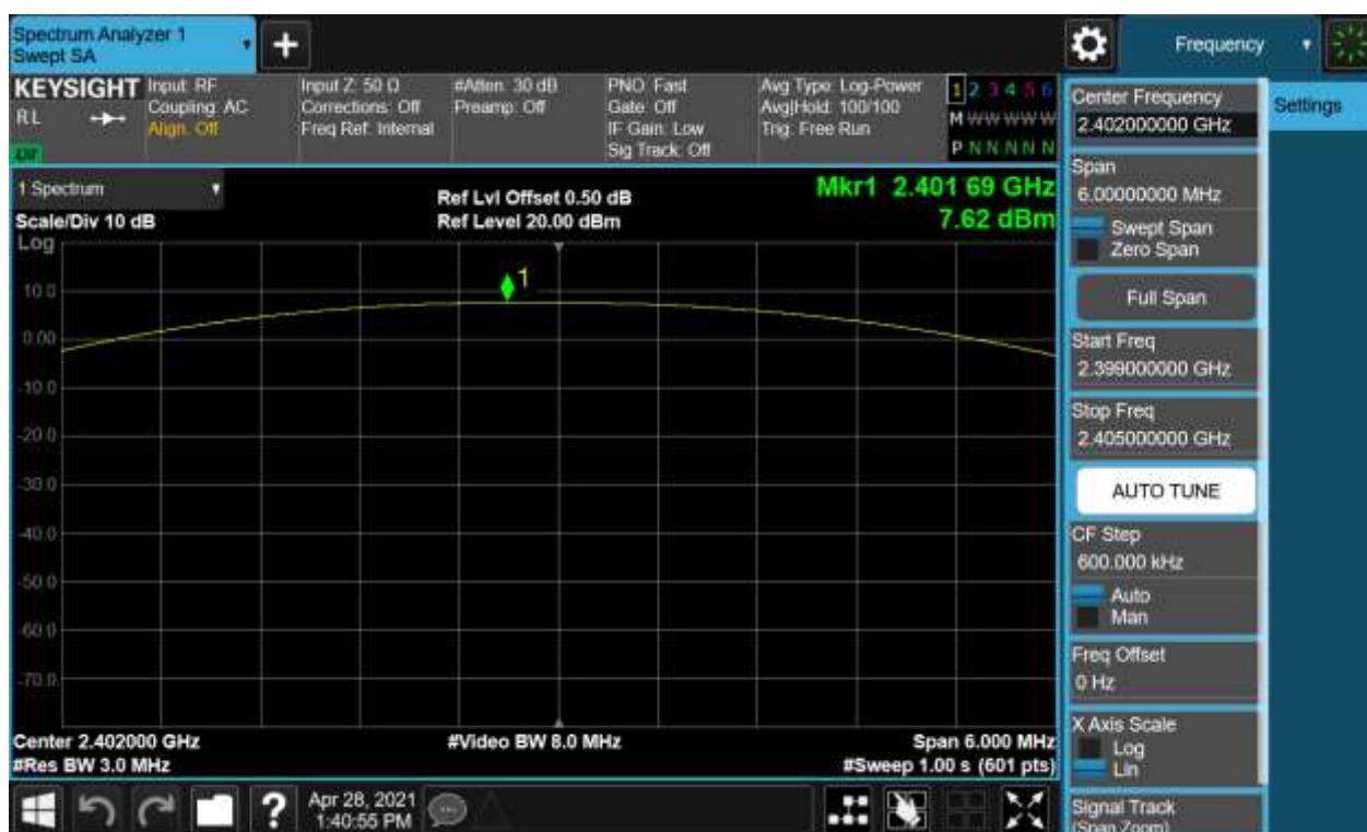
Figure 2: External Module-Maximum Conducted Output Power, 2402MHz, GFSK
