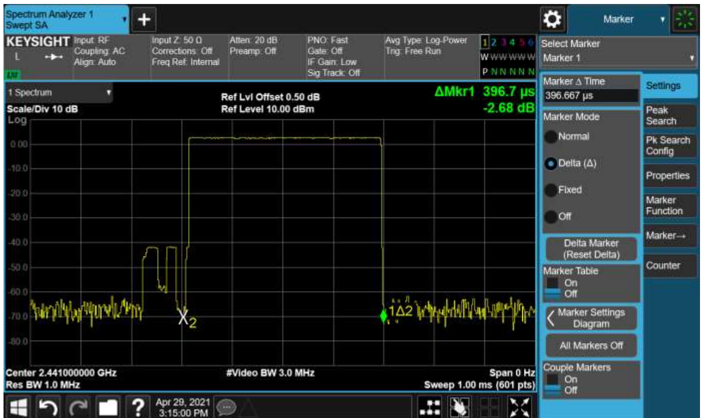
Figure 24: Internal Module-Time of Occupancy, 2441MHz, GFSK DH1
