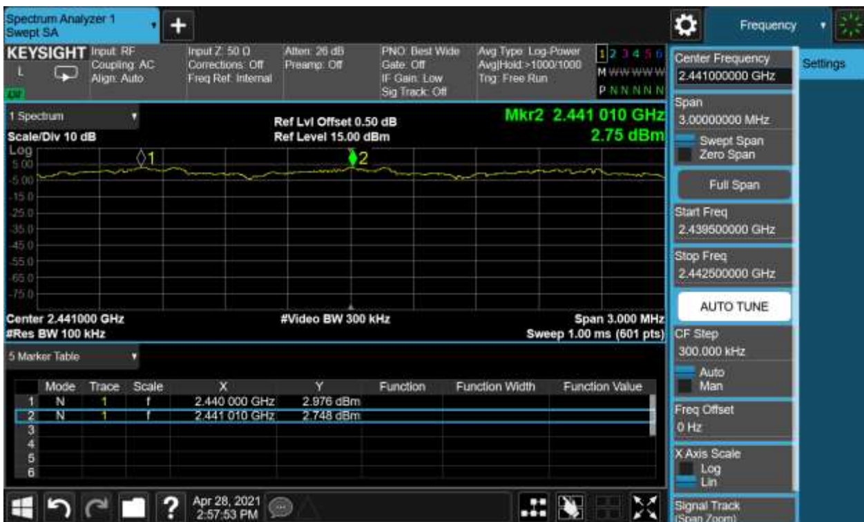
External Module-Hopping Frequency Separation, Hopping Mode, 8DPSK
