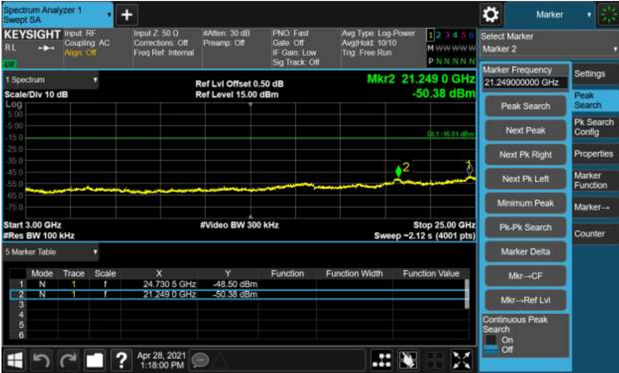
Figure 17: External Module -Conducted Spurious Emission & Authorized-band band-edge, 2441MHz, 8-DPSK Carrier Level
