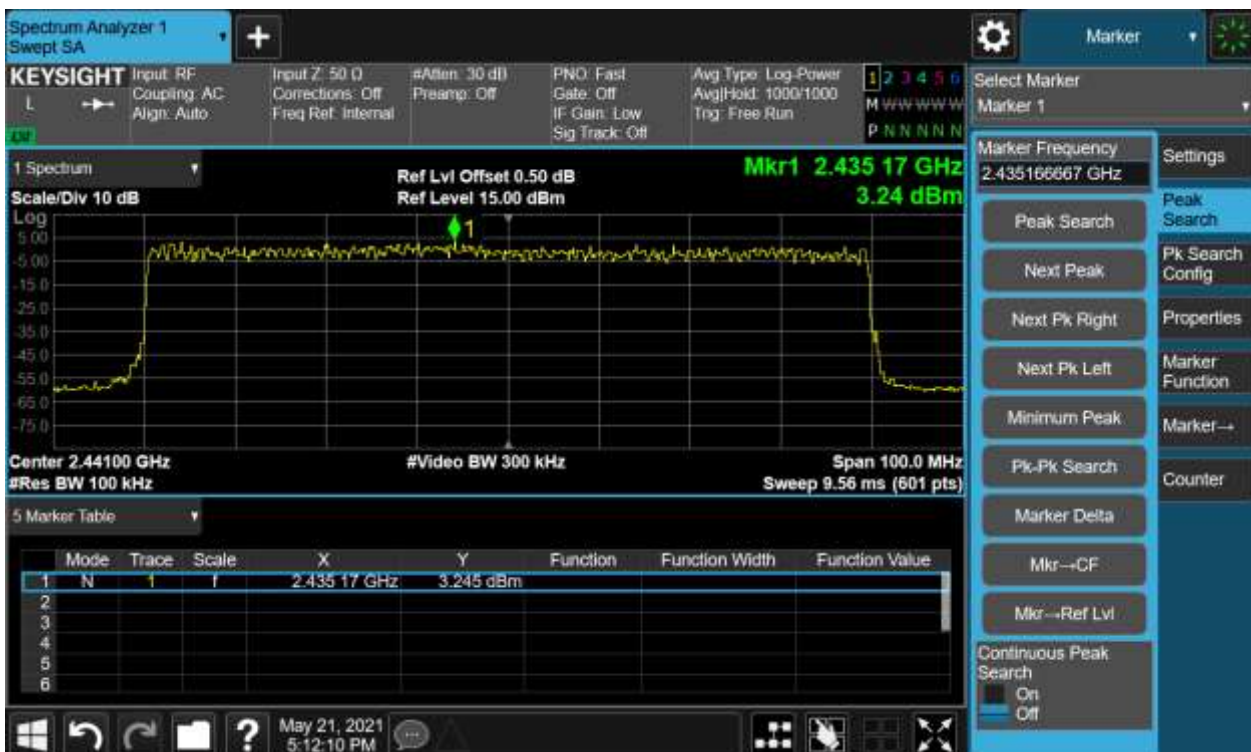
Figure 19: External Module -Conducted Spurious Emission & Authorized-band band-edge, Hopping mode, 8-DPSK Carrier Level
