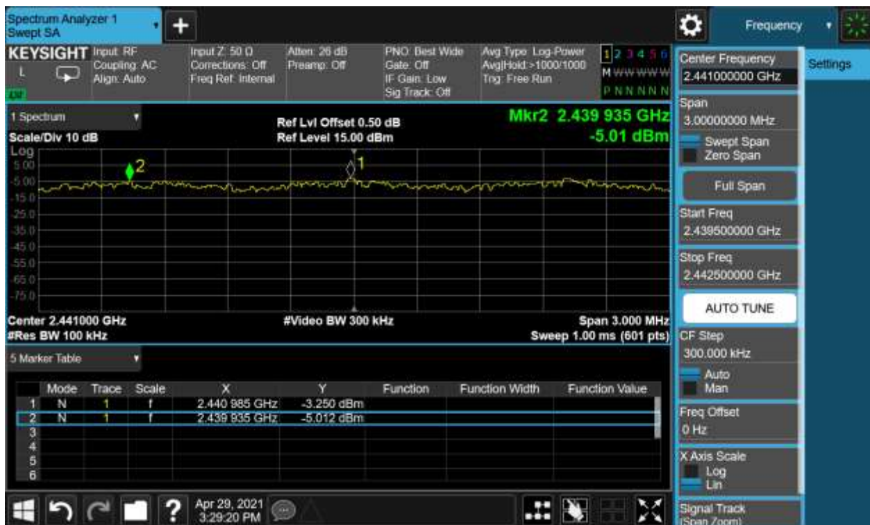
Internal Module-Hopping Frequency Separation, Hopping Mode, 8DPSK
