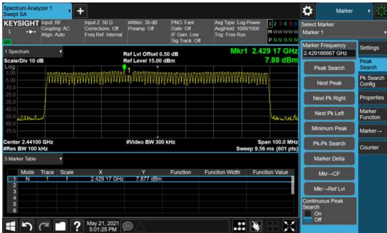
Figure 19: External Module -Conducted Spurious Emission & Authorized-band band-edge, Hopping mode, GFSK
