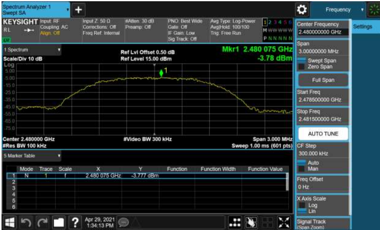
Figure 10: Internal Module-Conducted Spurious Emission & Authorized-band band-edge, 2480MHz, 8-DPSK Carrier Level
