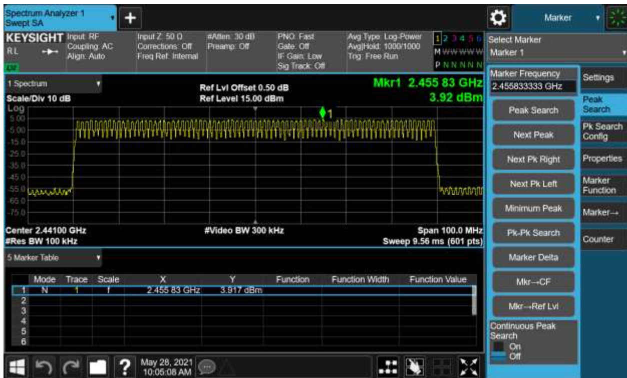
Figure 11: Internal Module-Conducted Spurious Emission & Authorized-band band-edge, Hopping Mode, GFSK
