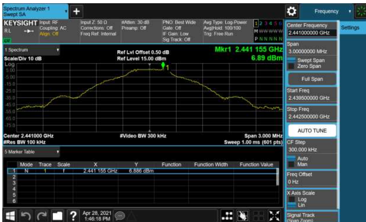
Figure 14: External Module -Conducted Spurious Emission & Authorized-band band-edge, 2441, GFSK Carrier Level
