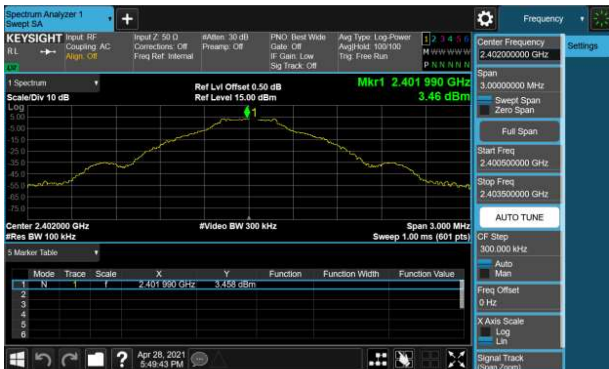
Figure 5: Internal Module-Conducted Spurious Emission & Authorized-band band-edge, 2402MHz, GFSK Carrier Level
