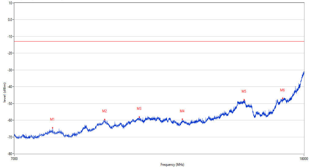
RSE Test case_CE FCC PART22&24&27_FCC GSM&CDMA&LTE&WCDMA 7-18G
