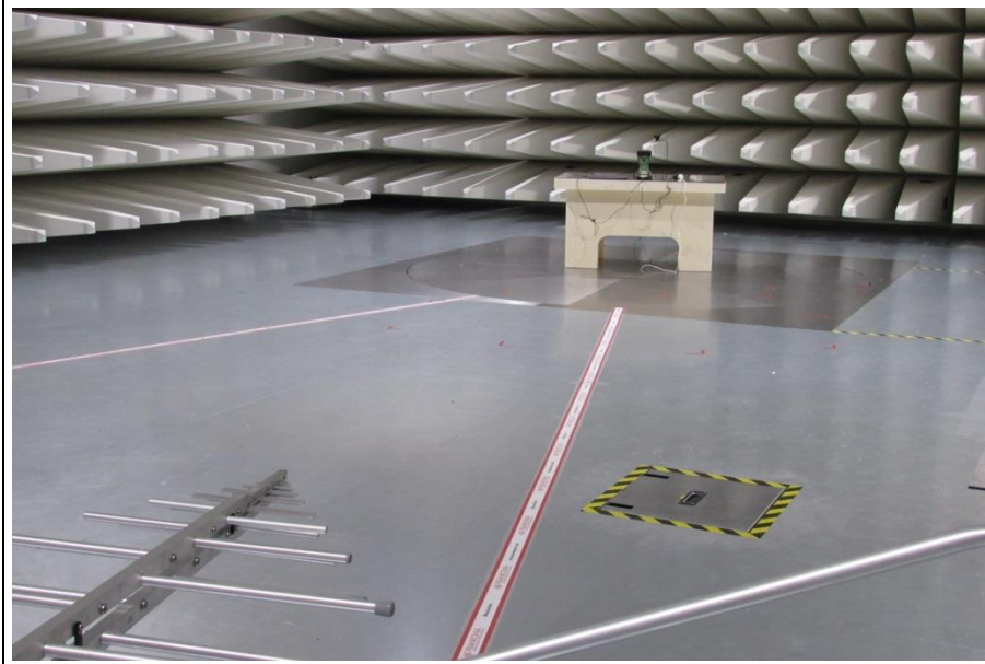
Test Setup : Radiated Emissions Docking Station
