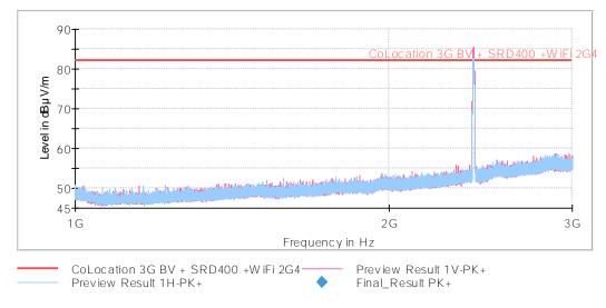
Settings: RBW = 1 MHz / VBW = 3 MHz / Sweep Time = 1s / Sweep points = 32000 The peak above the limit is the WLAN 2.4 GHz (2412 MHz) carrier frequency.
