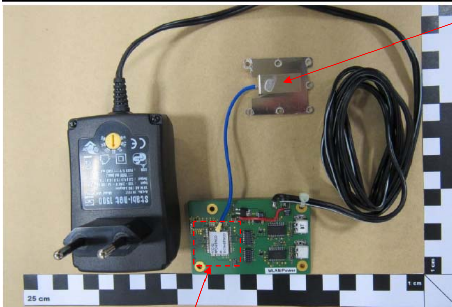
TiWi-BLE module mounted on evaluation board, power supply and antenna
