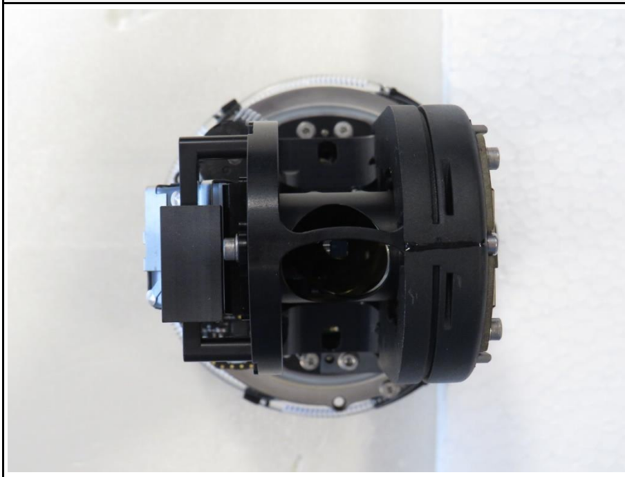
LASER SCANNER TOP SIDE
