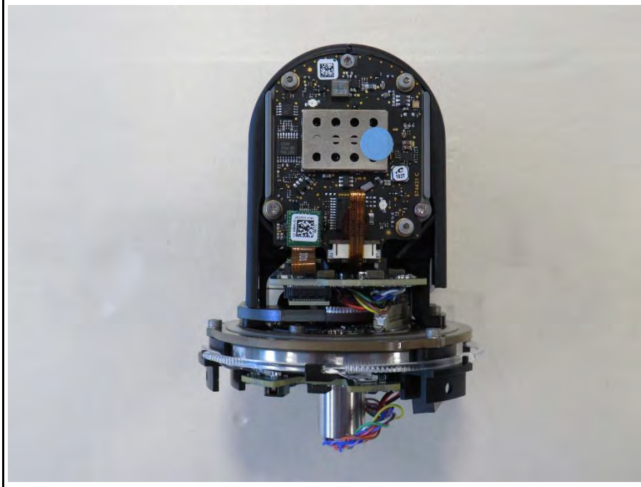
LASER SCANNER FRONT SIDE
