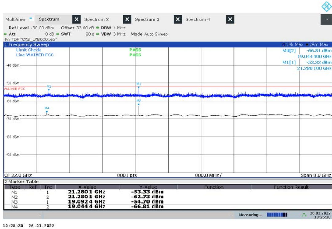
Plot no. 30: radiated emissions 18 GHz – 26.5 GHz, hor./vert. polarization, cw high
