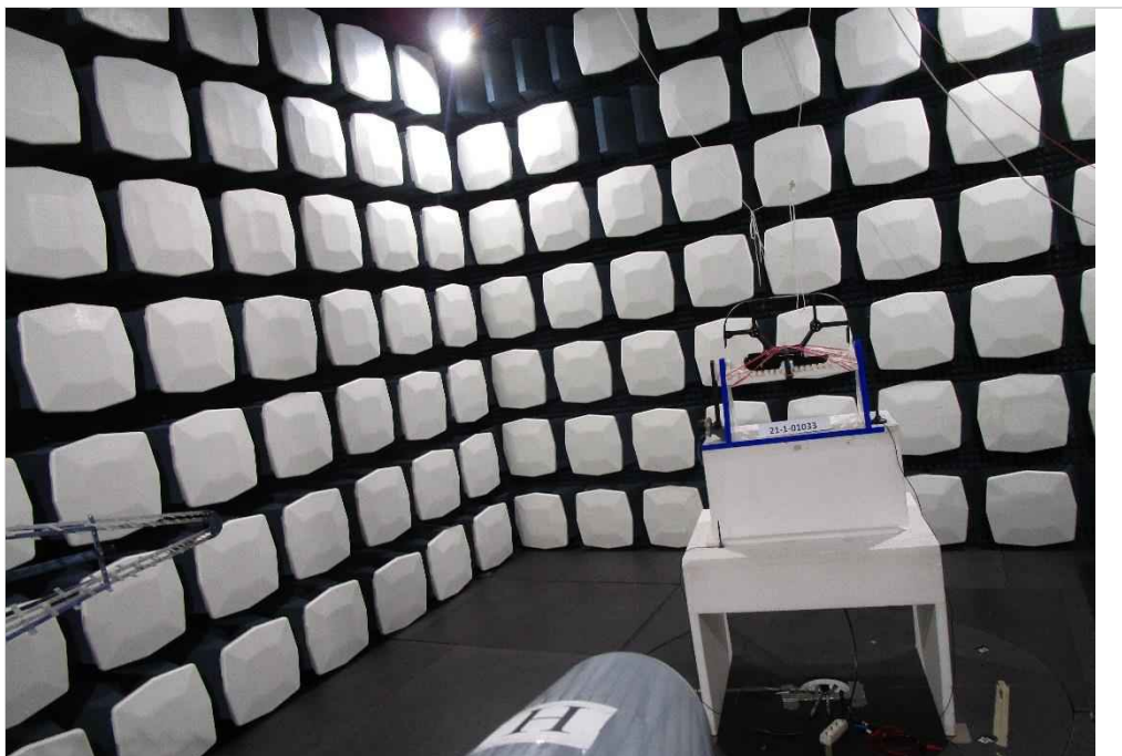
Photograph 2: EUT test setup in the fully anechoic chamber, overview_EUT elevation 0°
