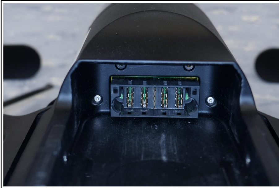
EUT battery port
