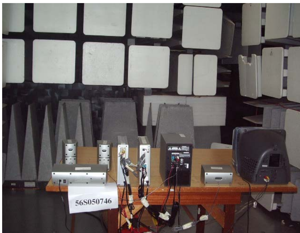
Radiated Emissions Test Setup (Front View)
