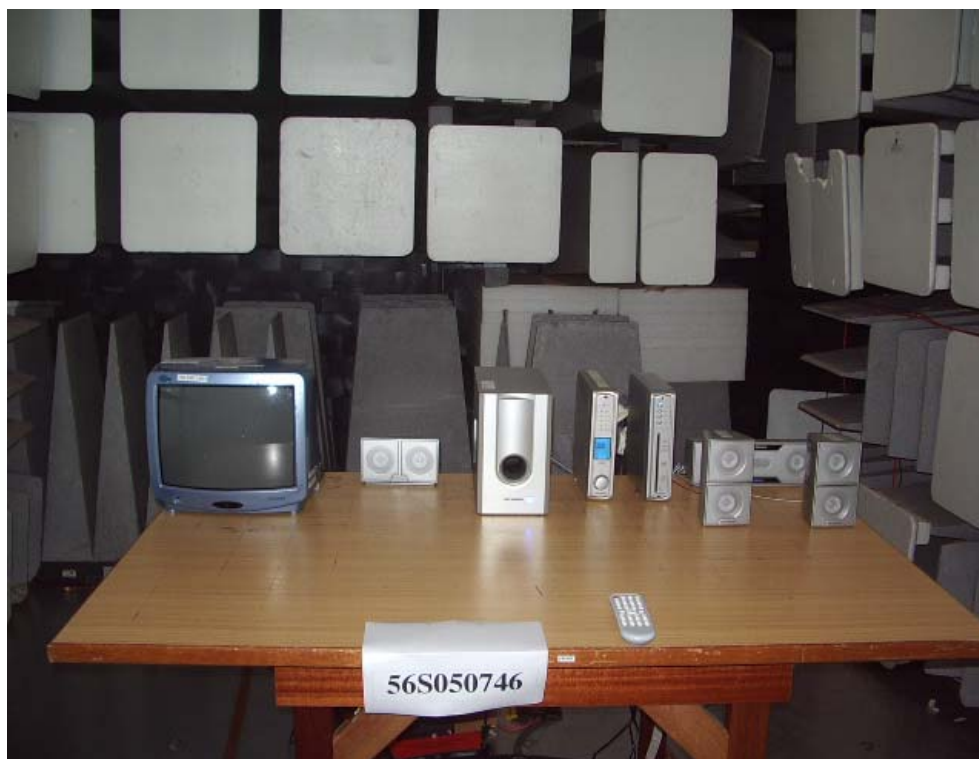
Radiated Emissions Test Setup (Front View)
