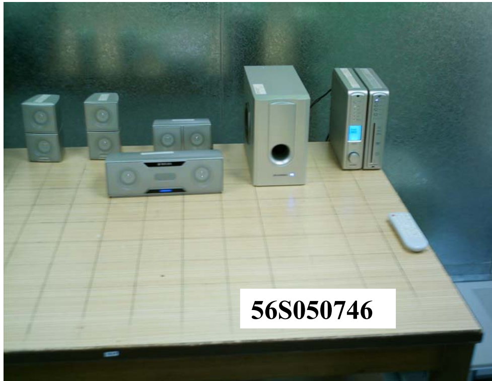
Conducted Emissions Test Setup (Front View)
