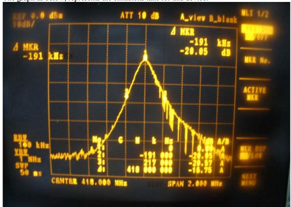
Bandwidth is determined at the points 20~dB down from the modulated carrier is 408KHz, it's less than the limit: 0.25% of the center frequency=1.02MHz
