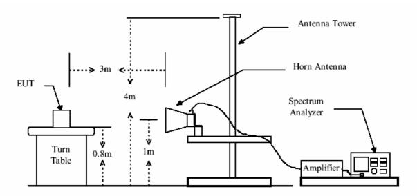
**Test Procedure:** The procedure uesd was ANSI Standard C63.4-2001. The receive was scanned from 30MHz to 5.0GHz. When an emission was found, the table was roated to produce the maximum signal strength. An initial pre-scan was performed for in peak detection mode using the receiver. The EUT was measured for both the Horizontal and Vertical polarities and performed a pre-test three orthogonal planes.
