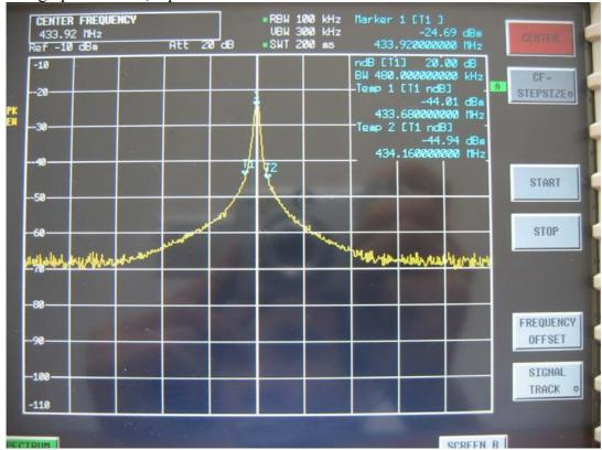
Bandwidth is determined at the points 20 dB down from the modulated carrier is 480 KHz, it's less than the limit: 0.25% of the center frequency = 1.08 MHz.
