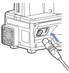
To remove the adapter, pull it out while pressing on the button at the top.
