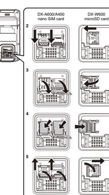
Even when not using a microSD or nano SIM card, be sure to close and lock the slot cover(s). NOTICE The slot cover(s) may be damaged if unlocked
