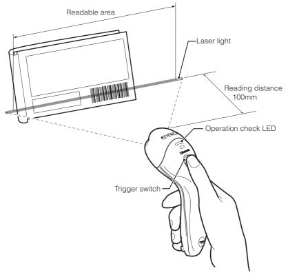
$oldsymbol{3}$  Once scanning is complete, the white LED lights up  $oldsymbol{\bigcirc}$  , a beep will sound once  $\Box \subset$  , and data is transmitted to your computer.
