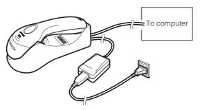
Charging is complete once the yellow LED stops blinking A full charge takes approximately 4 hours.
