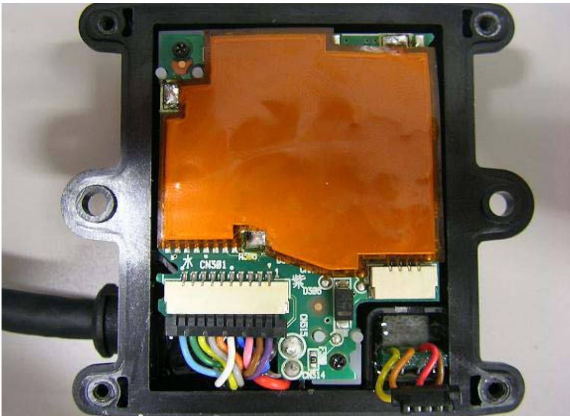
Internal View of RFID with Shield
