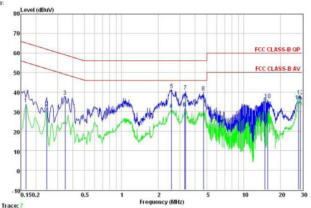
: CCIS Conducted Test Site : FCC CLASS-B QP LISN LINE Site Condition
