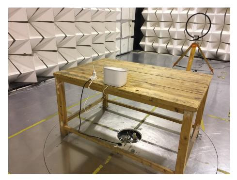
Test frequency from 30 MHz to 1 GHz
