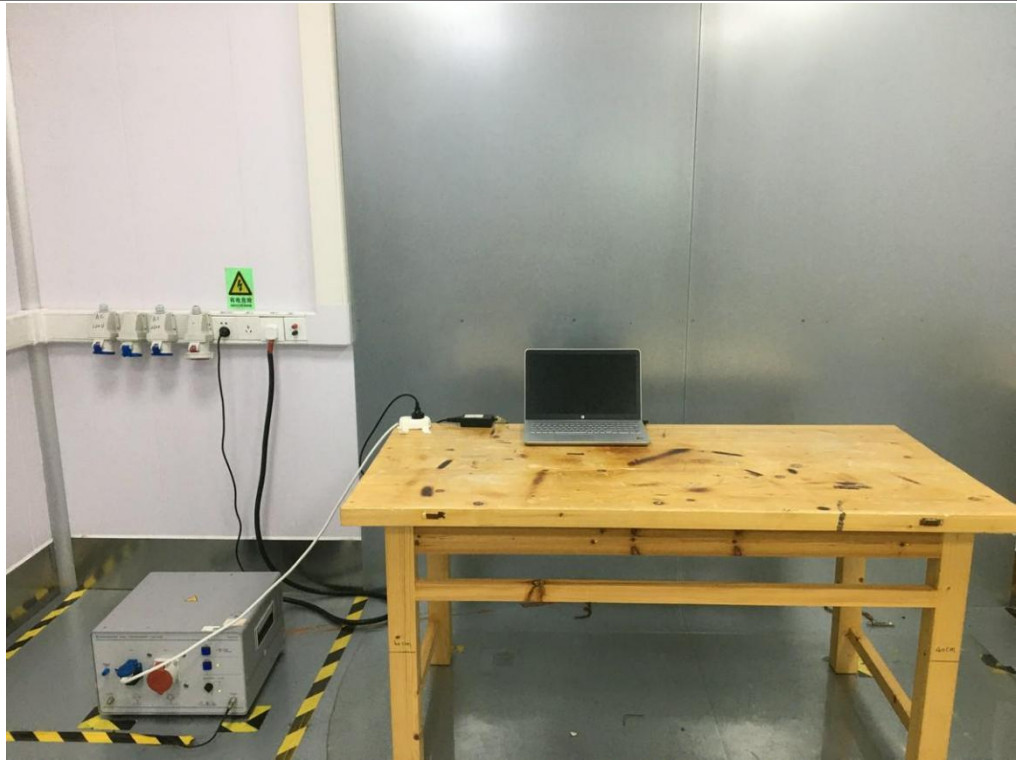
Conducted Emission at AC power line
