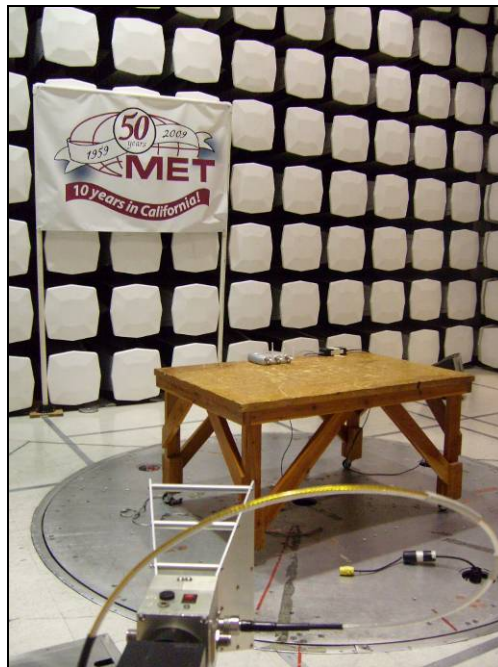
Photograph 6. Radiated Emission Test Setup 1 GHz – 6 GHz
