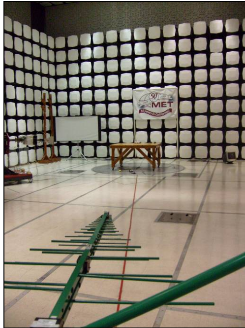
Photograph 5 Radiated Emission Test Setup 30 MHz – 1 GHz
