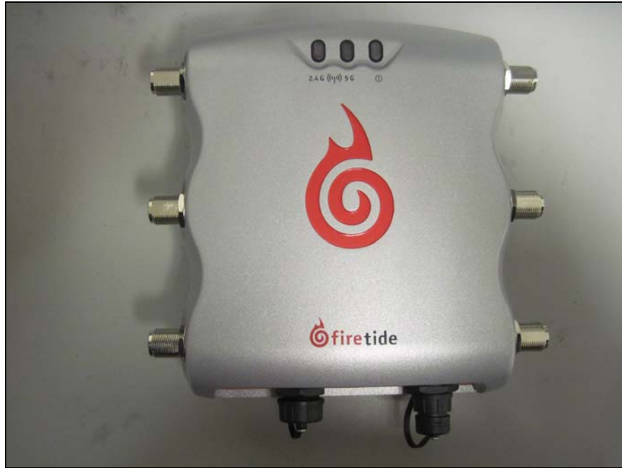
Photograph 1. Firetide, Inc. Firetide Indoor and Outdoor MIMO Access Points, Front View
