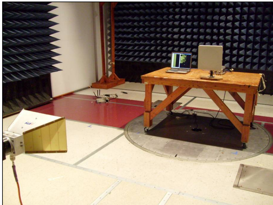
Photograph 9. Test Equipment and Setup for Various Radiated Measurements, 19 dBi Panel
