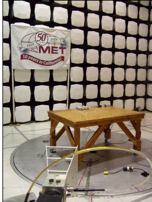
Photograph 6. Radiated Emission Test Setup 1 GHz – 6 GHz
