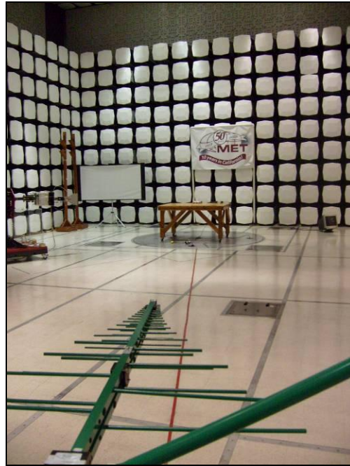
Photograph 5 Radiated Emission Test Setup 30 MHz – 1 GHz
