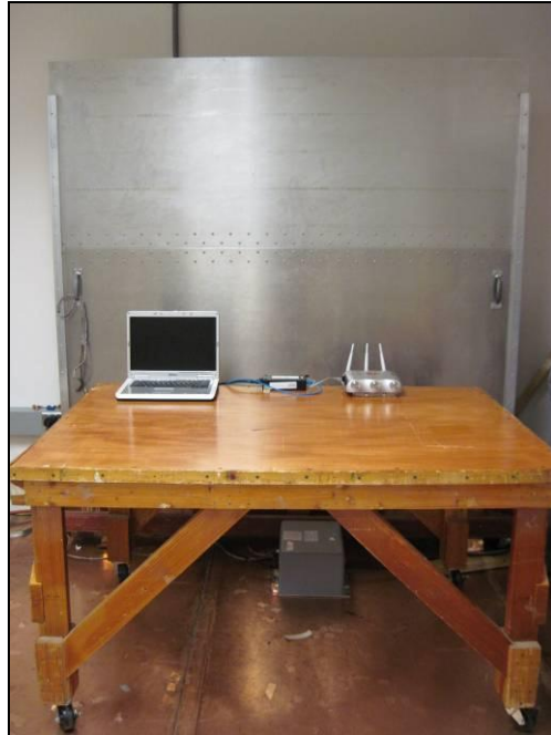
Photograph 3. Conducted Emissions, Test Setup 1
