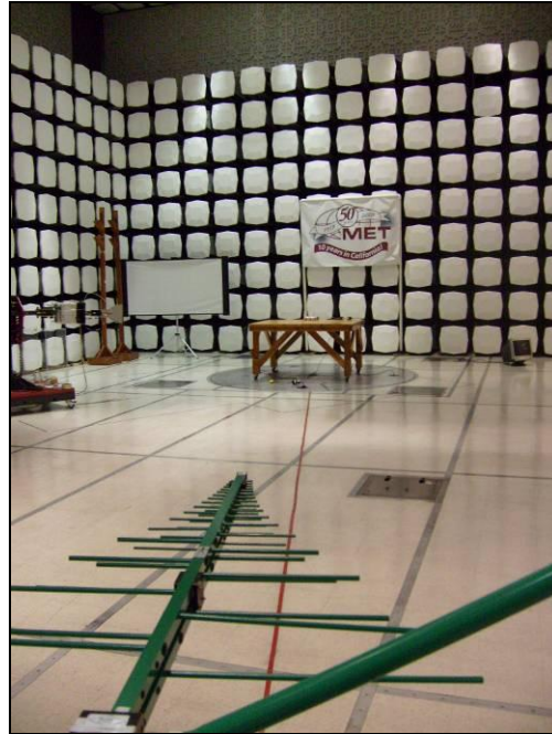
Photograph 5. Radiated Emission, Test Setup, 30 MHz – 1 GHz
