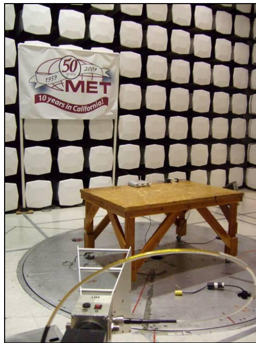
Photograph 6. Radiated Emission, Test Setup, 1 GHz – 6 GHz
