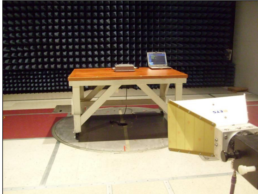
Photograph 8. Test Equipment and Setup for Various Radiated Measurements – 5 dBi Omni
