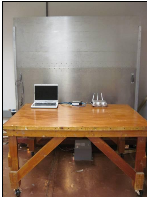
Photograph 7. Conducted Emissions, 15.207, Test Setup
