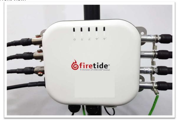
Note: Connect the lightning arrester of all antenna ports to protective ground.
