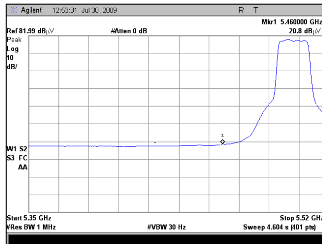
Plot 267. Restricted Band, 802.11a, 5460 Average, 19 dBi Panel
