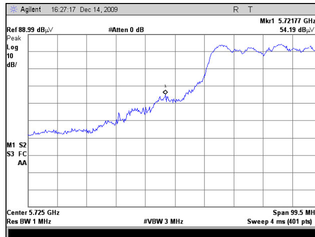
Plot 178. EIRP, 802.11n 40MHz, Low Channel, 5755 MHz, 9 dBi Omni
