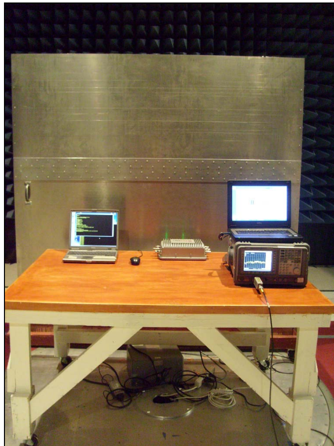
Photograph 5. Conducted Emissions, Test Setup
