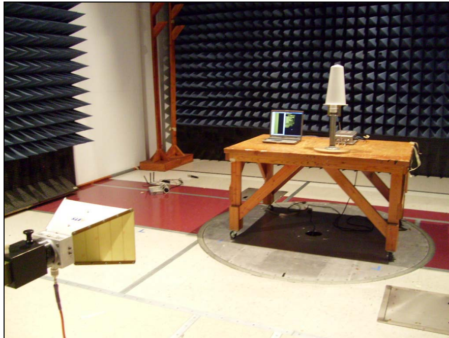
Photograph 6. Test Equipment and Setup for Various Radiated Measurements, 9 dBi Omni
