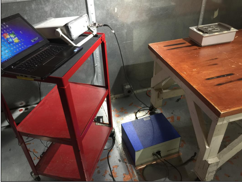
Photograph 7. Conducted Emissions, Test Setup
