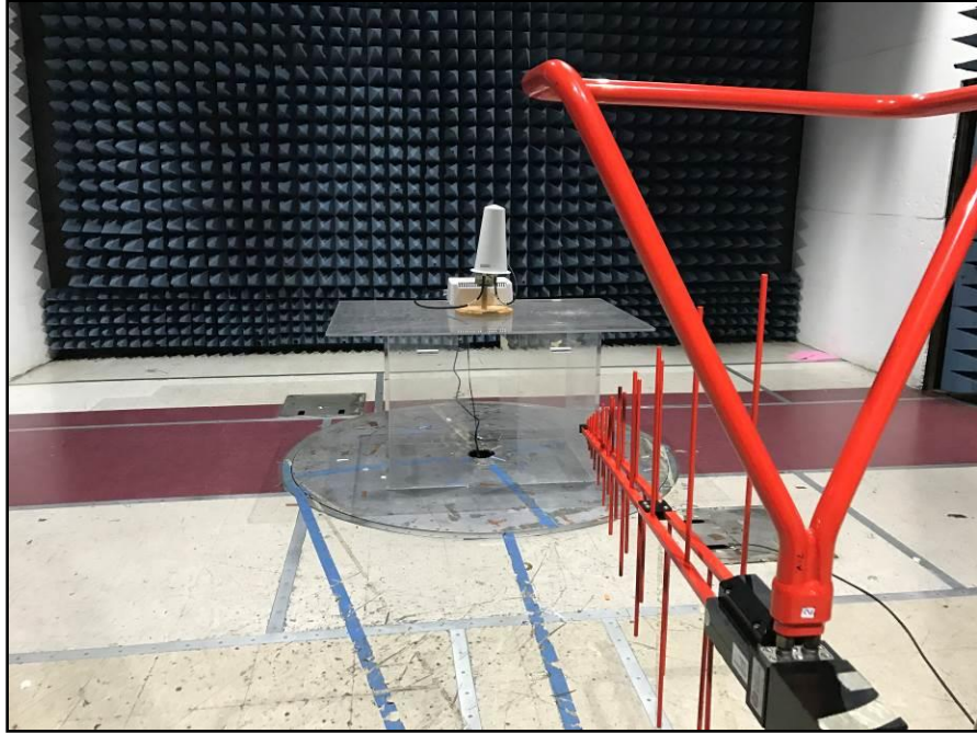
Photograph 1. Radiated Spurious Emissions, Test Setup, 30 MHz – 1 GHz, 9 dBi Antenna
