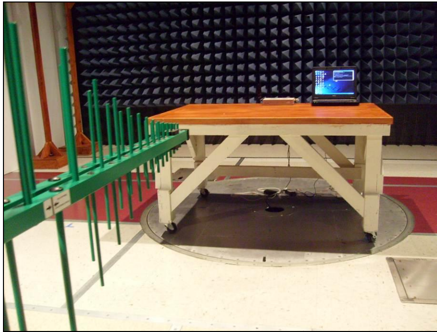
Photograph 3 Radiated Emission Test Setup 30 MHz – 1 GHz
