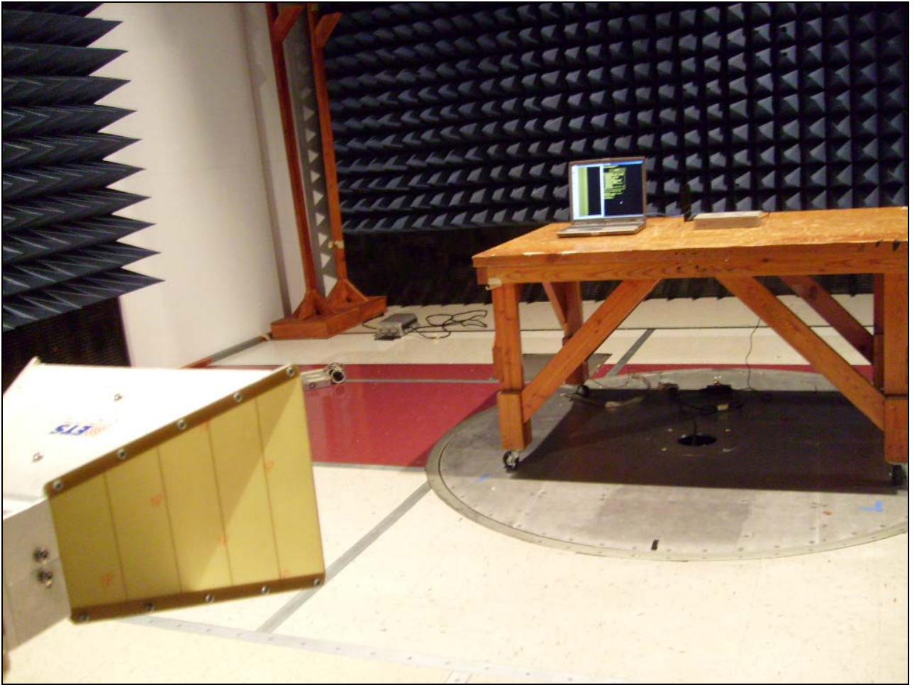
Test Equipment and Setup for Various Radiated Measurements – Combined Omni Antennas
