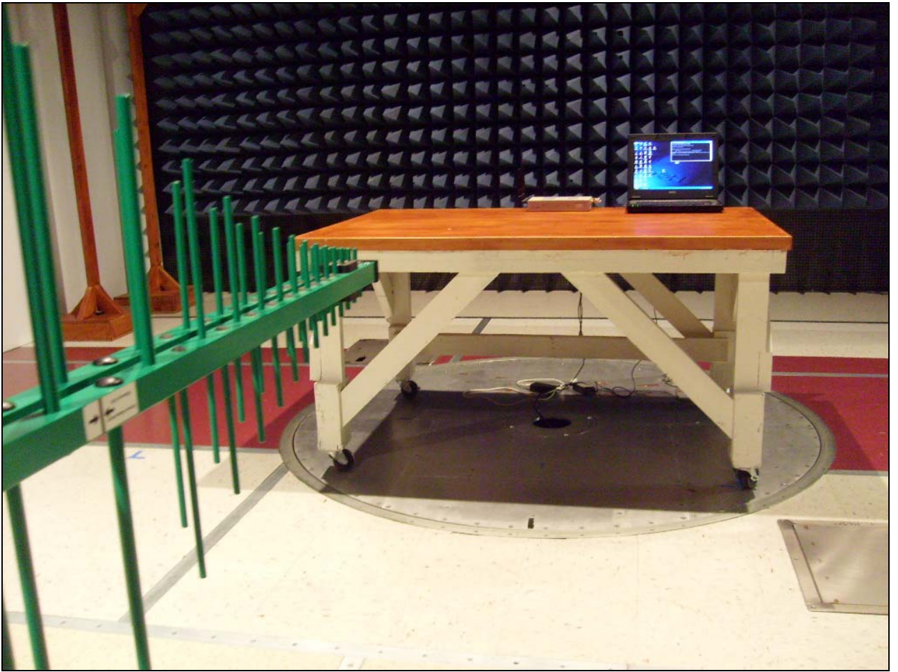
Radiated Emission, Test Setup, 30 MHz – 1 GHz
