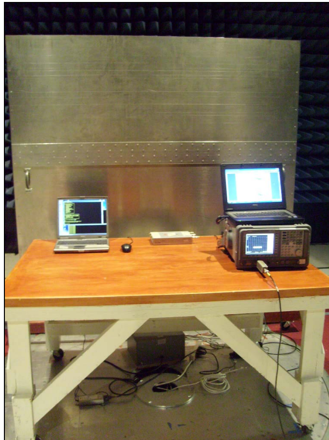
Photograph 2. Conducted Emissions Test Setup
