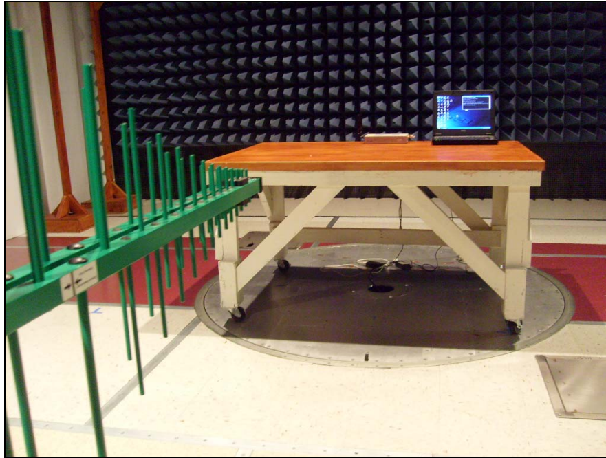
Photograph 3 Radiated Emission Test Setup 30 MHz – 1 GHz
