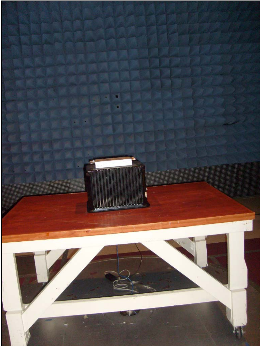
Photograph 1. Radiated Emission Spurious Test Setup, 1
