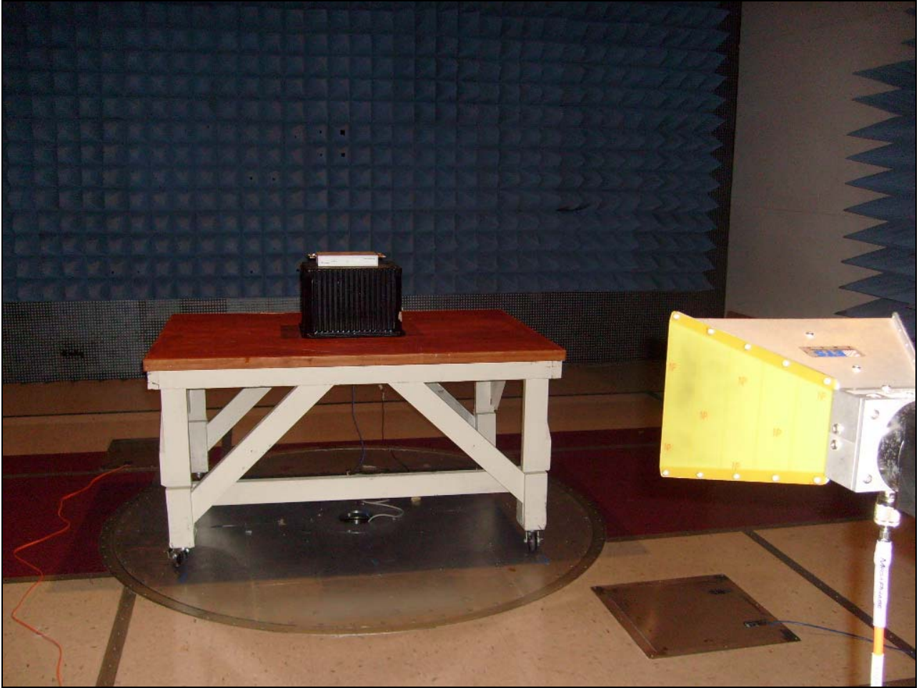
Photograph 3. Radiated Emission Spurious Test Setup, 3
