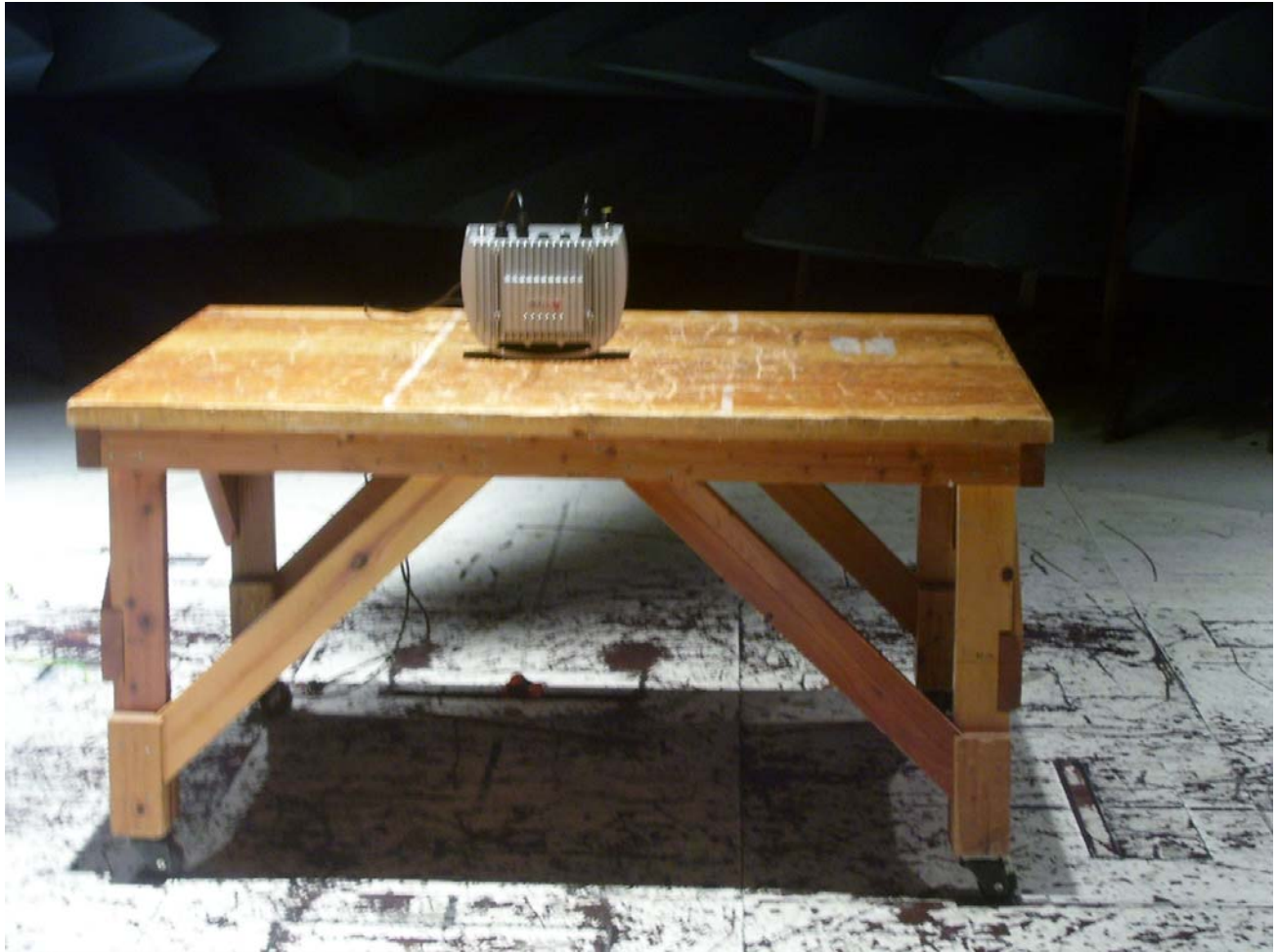
Photograph 4. Radiated Emission Spurious Test Setup
