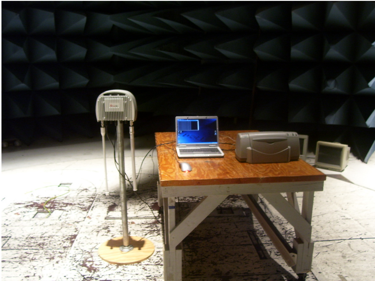
Photograph 3. Radiated Emission Limits Test Setup
