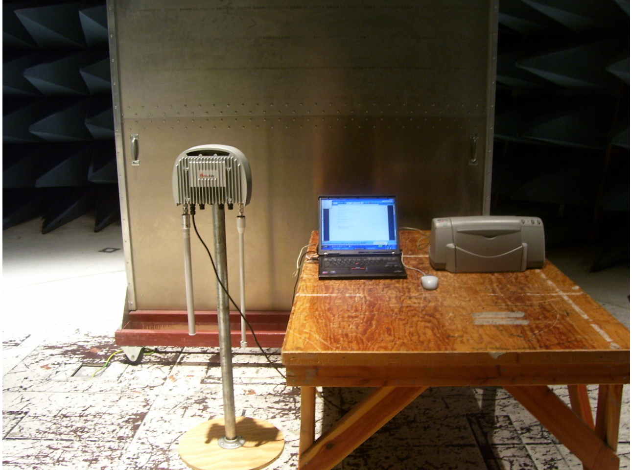
Photograph 4. Conducted Emissions Test Setup Photograph
