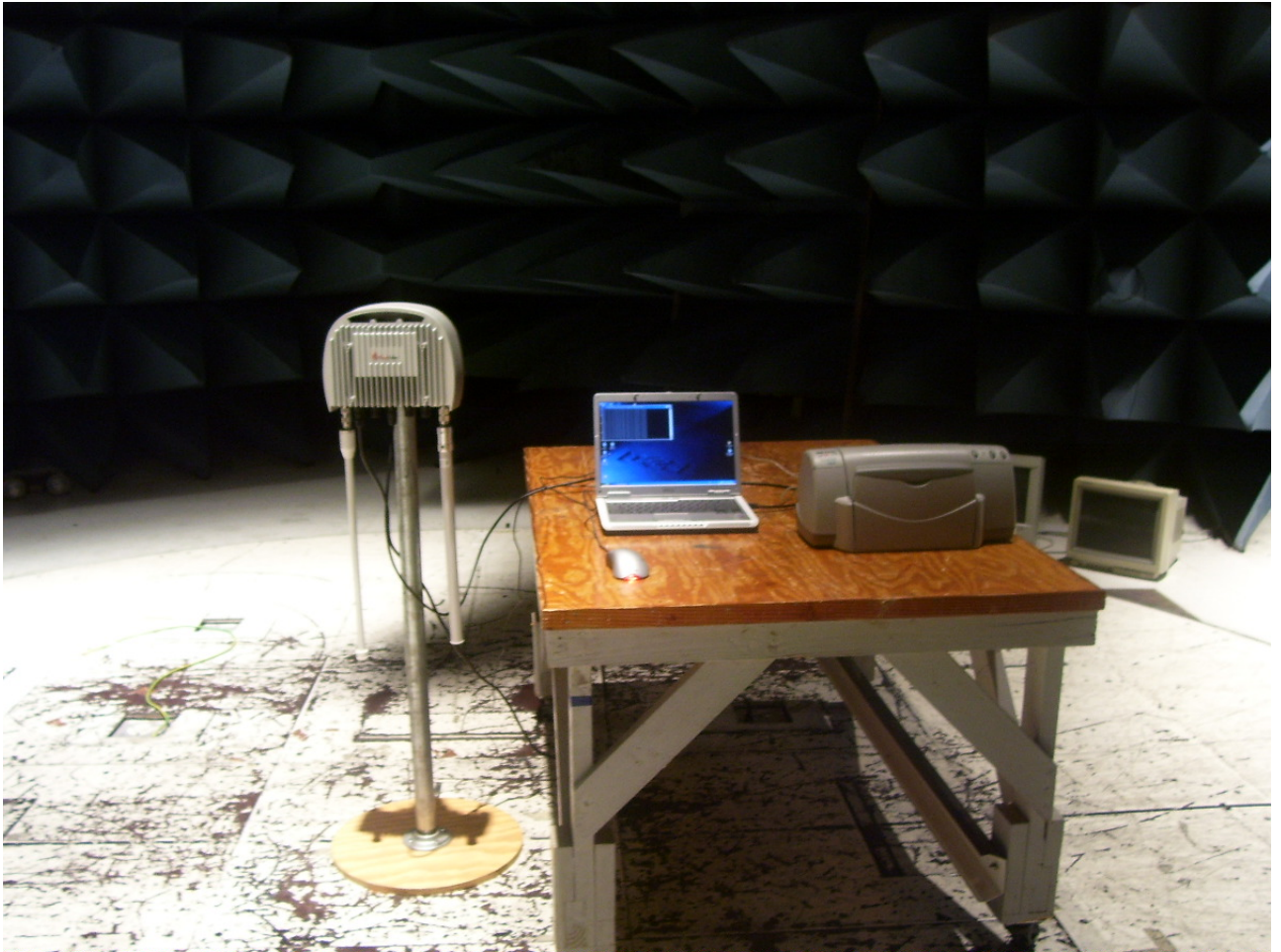
Radiated Emission Test Setup 30 MHz - 1 GHz
