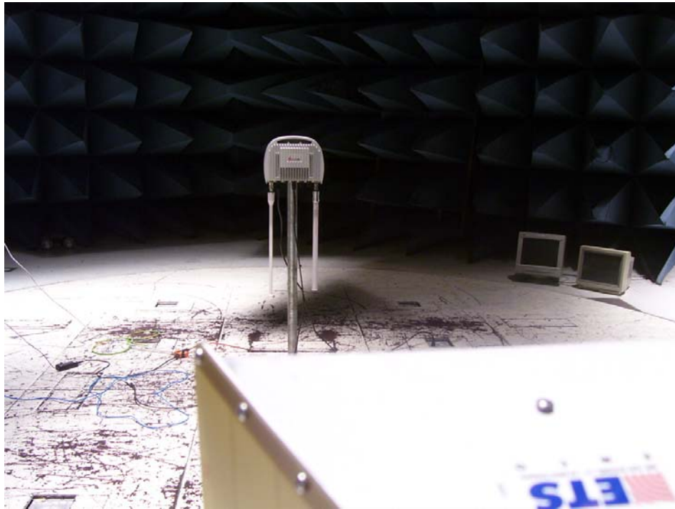
Photograph 2. Test Equipment and setup for various Radiated Measurements 10dbi Omni
