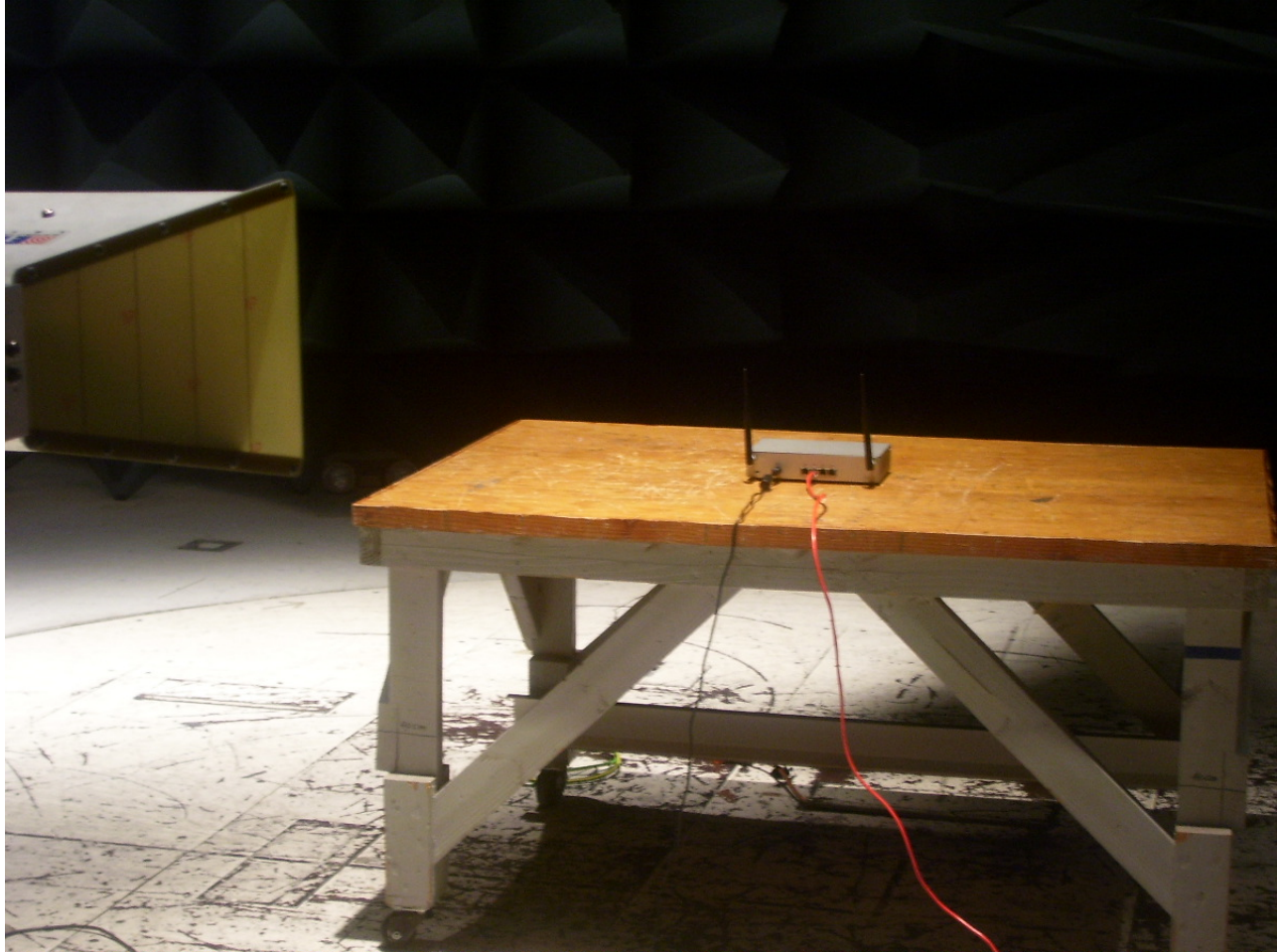
Photograph 4. Radiated Emission Spurious Test Setup
