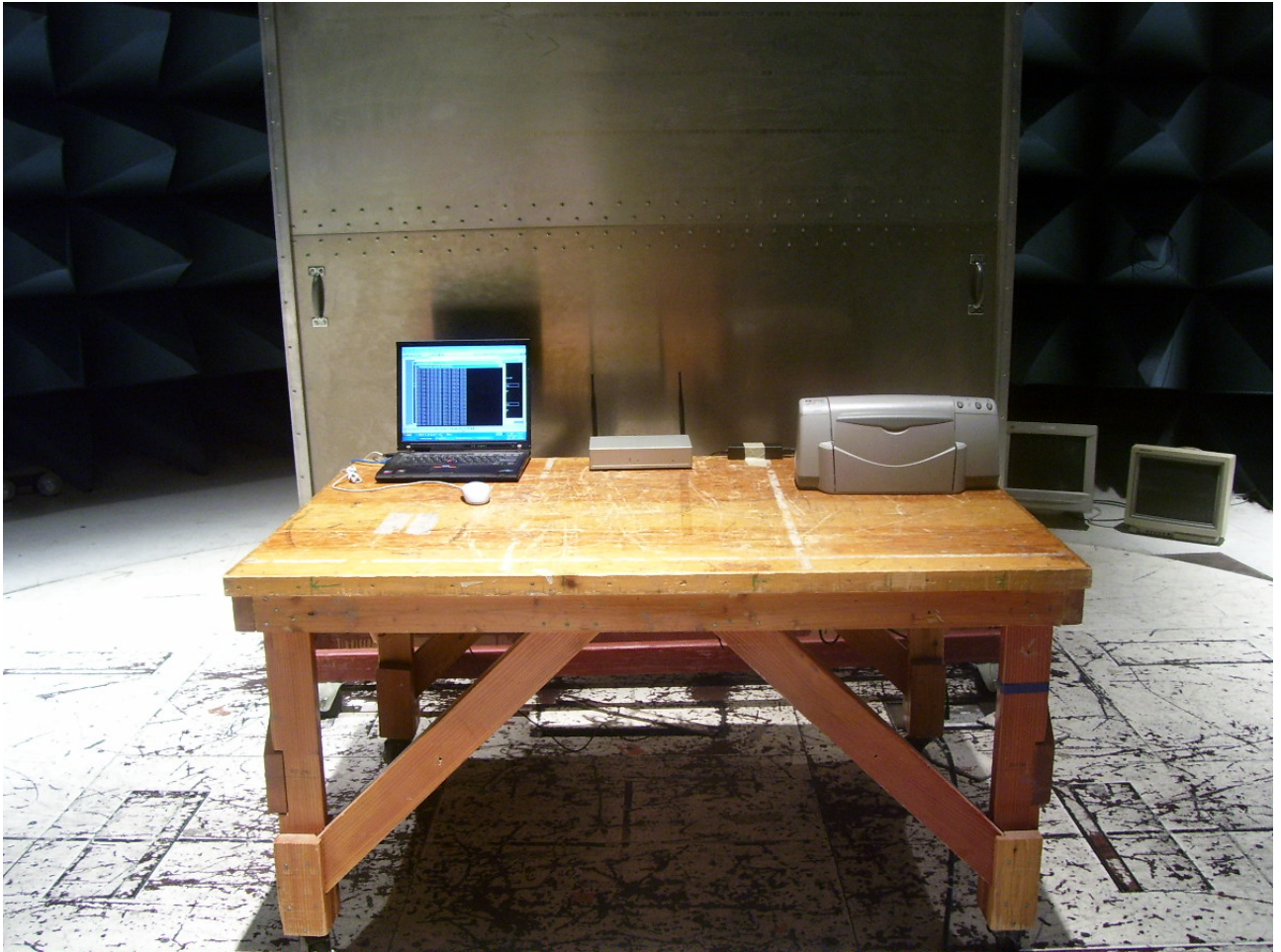
Conducted Emissions Test Setup
