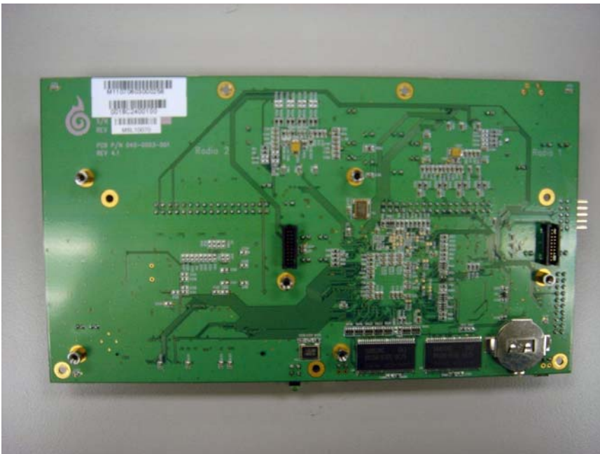
Solder side of Motherboard
