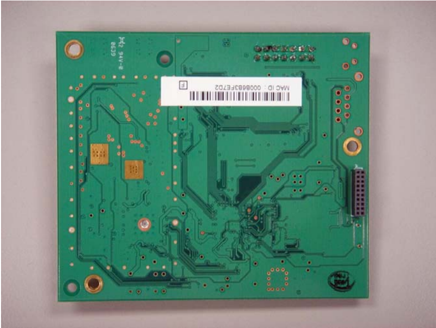
Solder side of Radio Card
