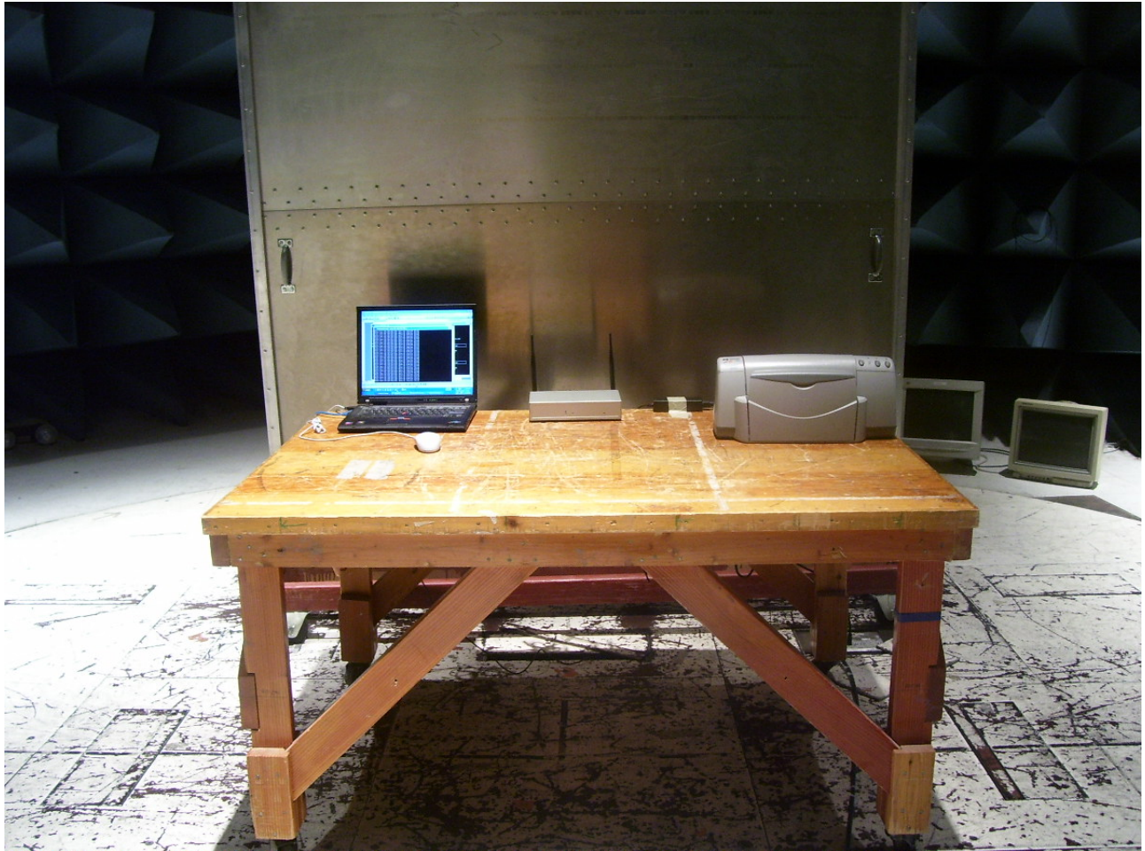
Photograph 2. Conducted Emissions Test Setup
