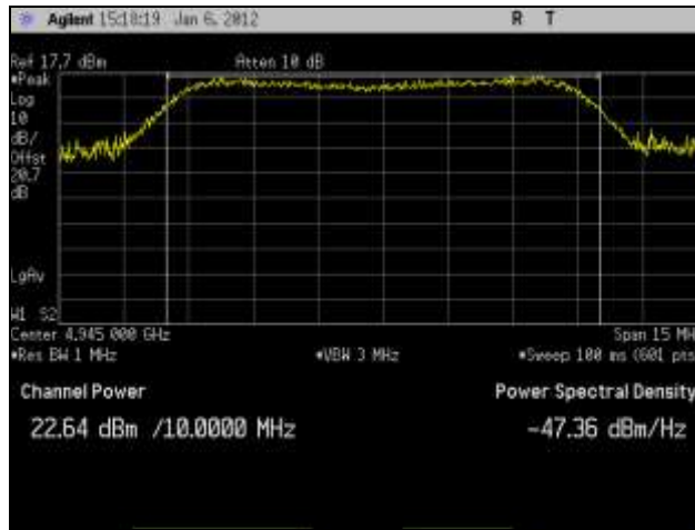
Plot 3. RF Power Output, Low Channel, 802.11n 10 MHz, Port 1
