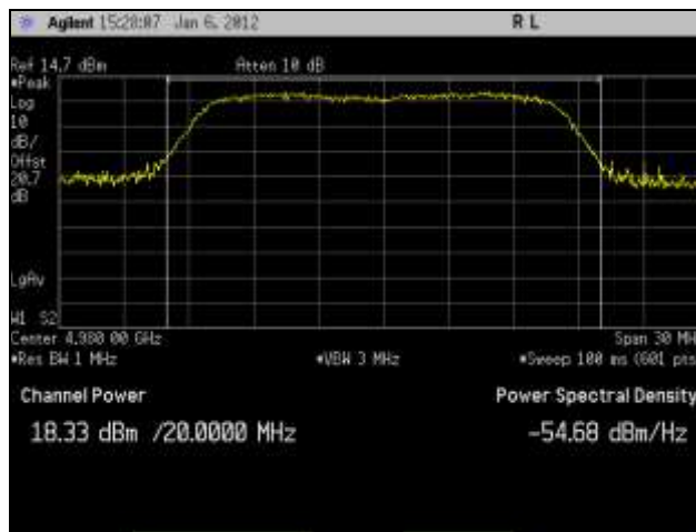
Plot 17. RF Power Output, High Channel, 802.11n 20 MHz, Port 3
