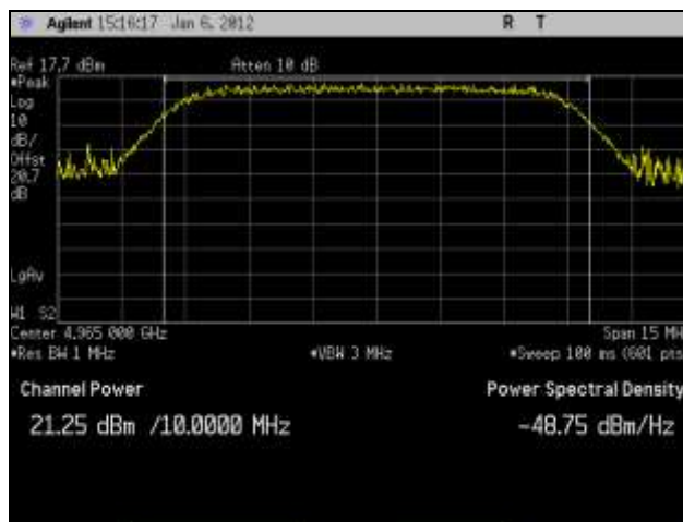
Plot 7. RF Power Output, Mid Channel, 802.11n 10 MHz, Port 2
