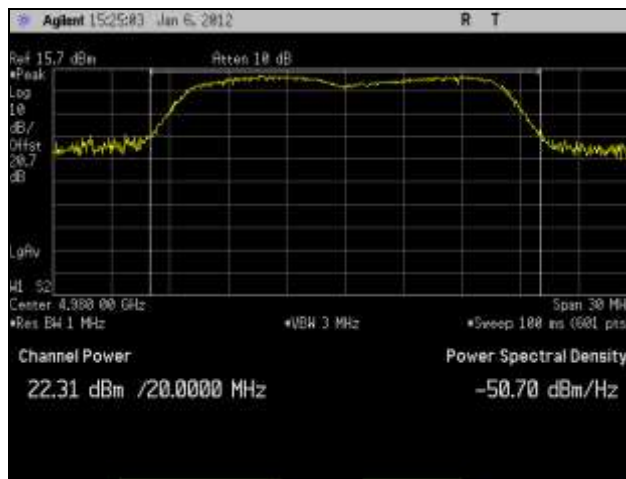
Plot 2. RF Power Output, High Channel, 802.11a
