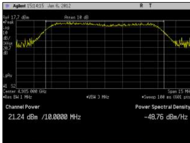
Plot 5. RF Power Output, High Channel, 802.11n 10 MHz, Port 1
