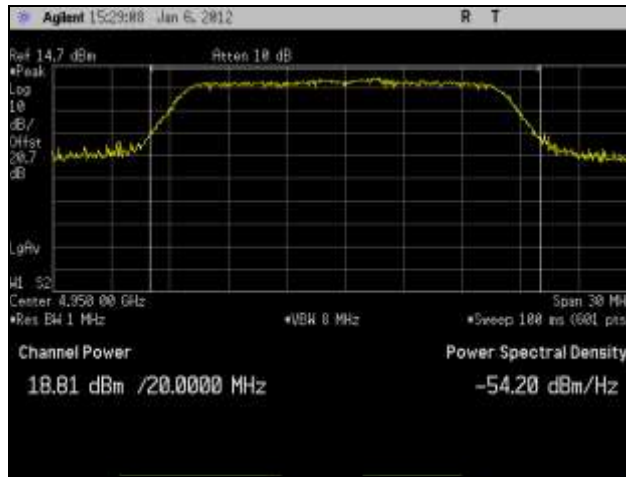
Plot 16. RF Power Output, Low Channel, 802.11n 20 MHz, Port 3
