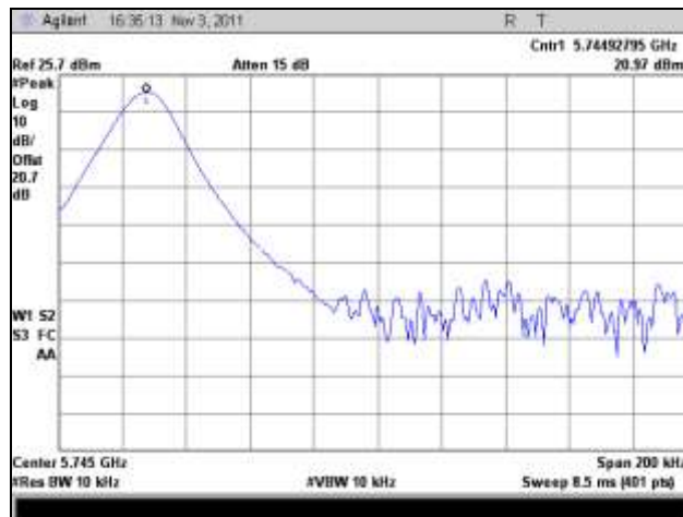
Plot 456. Frequency Stability, 5745 MHz, 10°C
