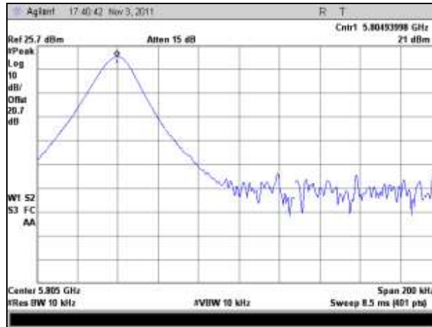
Plot 512. Frequency Stability, 5805 MHz, 50°C
