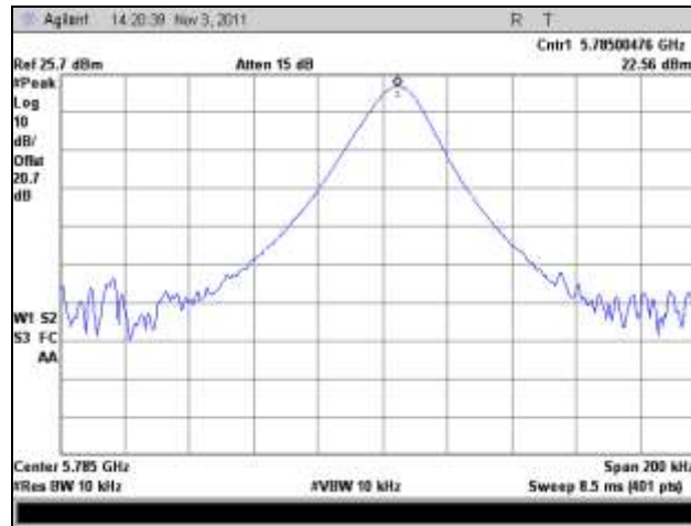
Plot 477. Frequency Stability, 5785 MHz, -40°C
