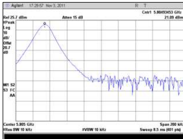
Plot 511. Frequency Stability, 5805 MHz, 40°C
