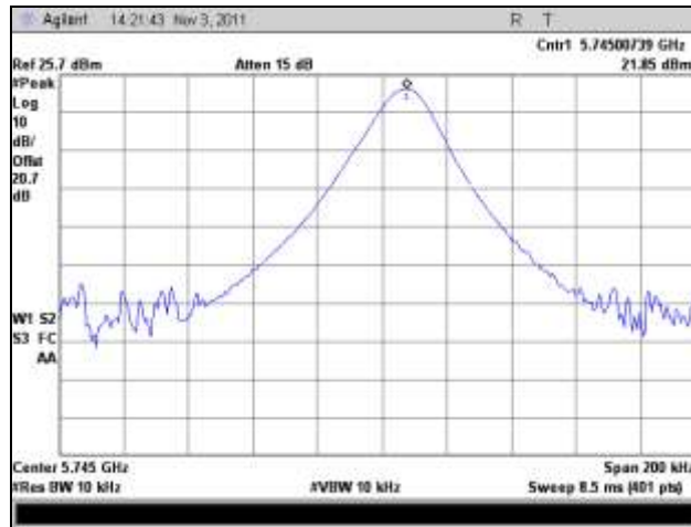
Plot 451. Frequency Stability, 5745 MHz, -40°C
