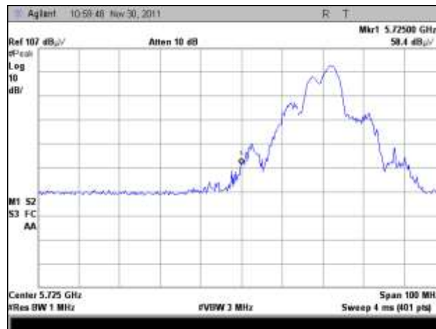
Plot 278. EIRP, 5725 MHz, Peak, 802.11n 10 MHz, 15 dBi Sector
