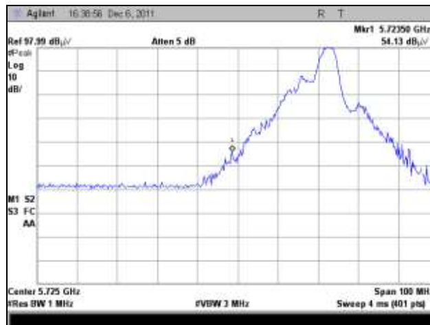
Plot 308. EIRP, 5725 MHz, Peak, 802.11n 10 MHz, 16 dBi Panel
