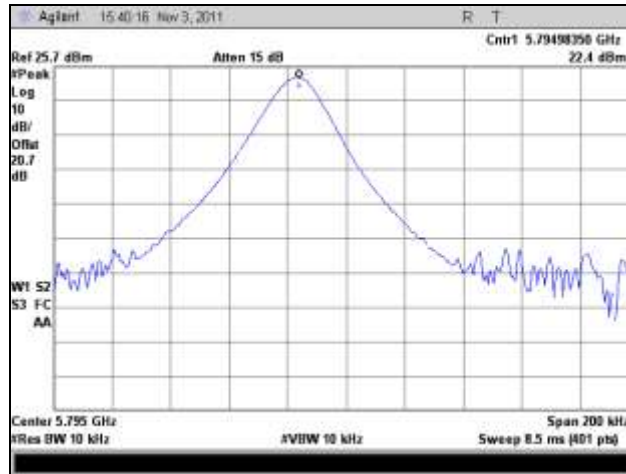
Plot 493. Frequency Stability, 5795 MHz, -10°C
