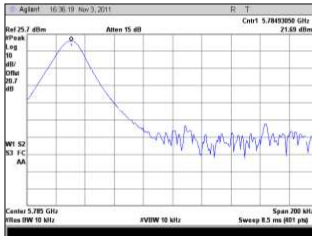
Plot 482. Frequency Stability, 5785 MHz, 10°C
