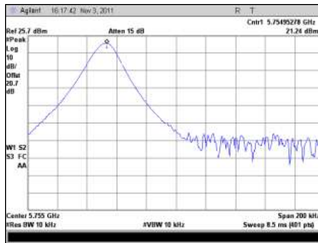
Plot 468. Frequency Stability, 5755 MHz, 0°C
