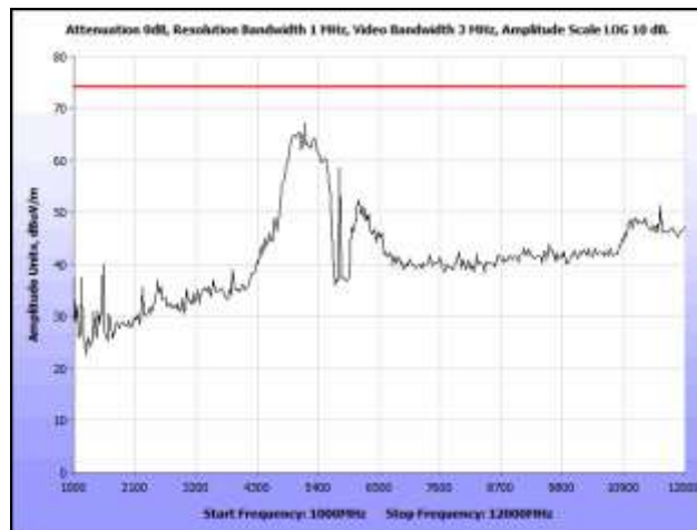
Plot 337. Restricted Band, Mid Channel, 1 GHz – 12 GHz, Peak, 802.11n 5 MHz, 9 dBi Omni
