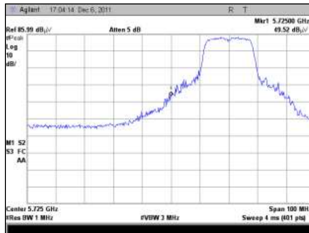
Plot 296. EIRP, 5725 MHz, Peak, 802.11a, 16 dBi Panel
