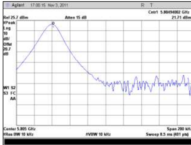
Plot 509. Frequency Stability, 5805 MHz, 20°C
