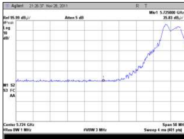
Plot 241. EIRP, 5725 MHz, Peak, 802.11n 5 MHz, 9 dBi Omni
