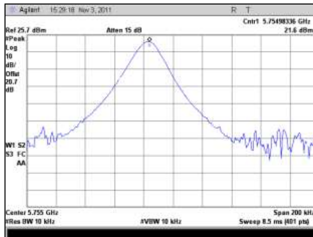
Plot 466. Frequency Stability, 5755 MHz, -20°C
