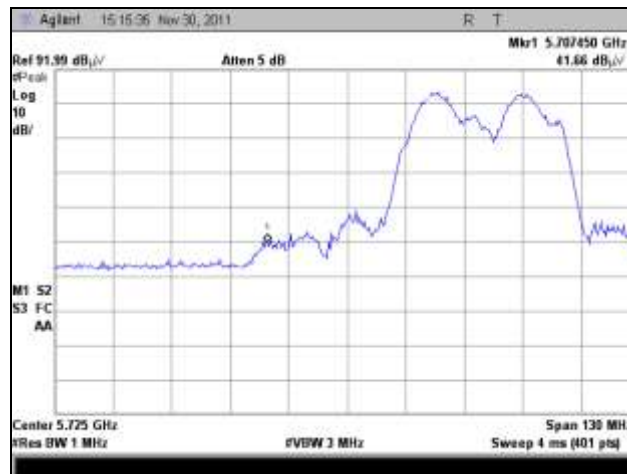
Plot 290. EIRP, 5725 MHz, Peak, 802.11n 40 MHz, 15 dBi Sector
