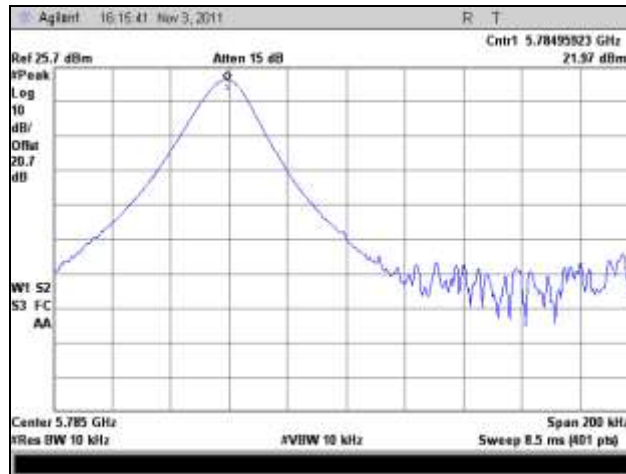
Plot 481. Frequency Stability, 5785 MHz, 0°C
