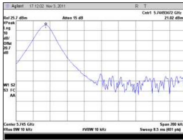
Plot 458. Frequency Stability, 5745 MHz, 30°C
