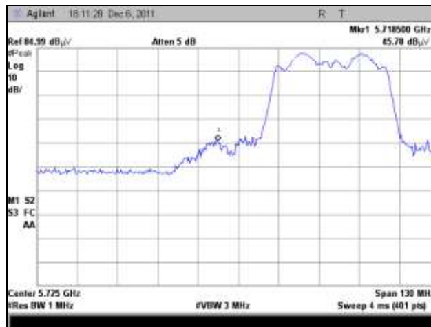
Plot 320. EIRP, 5725 MHz, Peak, 802.11n 40 MHz, 16 dBi Panel
