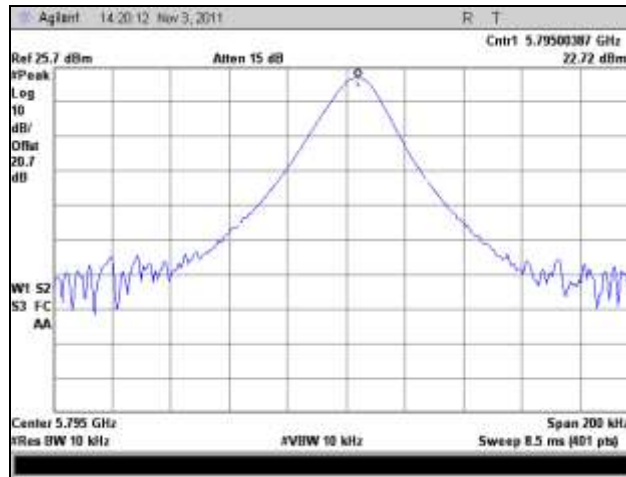
Plot 490. Frequency Stability, 5795 MHz, -40°C
