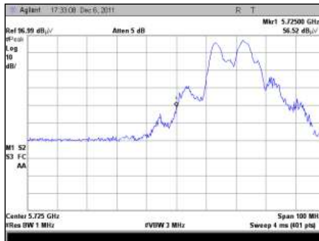
Plot 314. EIRP, 5725 MHz, Peak, 802.11n 20 MHz, 16 dBi Panel
