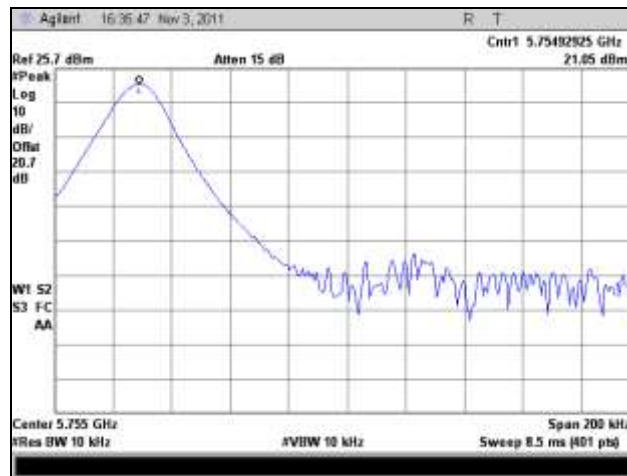
Plot 469. Frequency Stability, 5755 MHz, 10°C
