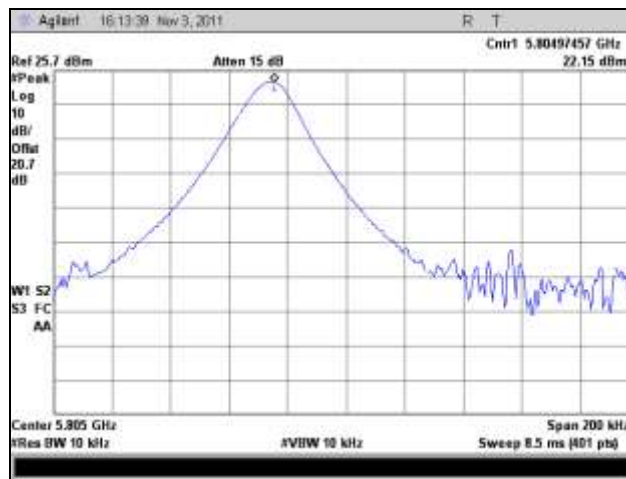
Plot 507. Frequency Stability, 5805 MHz, 0°C
