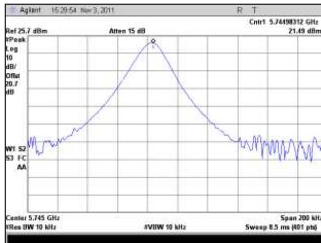
Plot 453. Frequency Stability, 5745 MHz, -20°C
