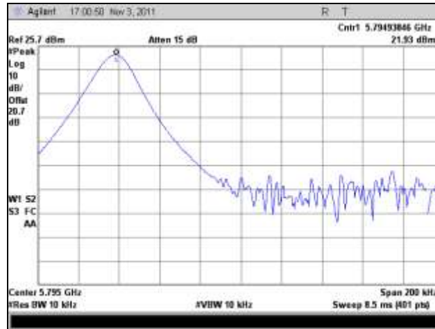
Plot 496. Frequency Stability, 5795 MHz, 20°C
