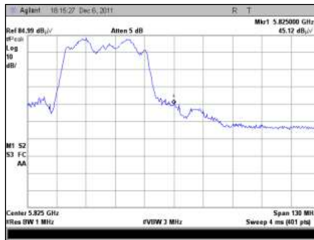
Plot 322. EIRP, 5825 MHz, Peak, 802.11n 40 MHz, 16 dBi Panel
