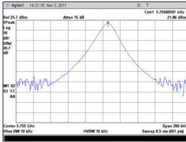
Plot 464. Frequency Stability, 5755 MHz, -40°C
