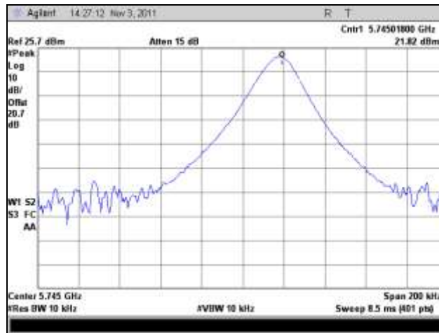
Plot 452. Frequency Stability, 5745 MHz, -30°C
