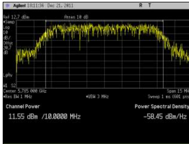
Plot 93. RF Power Output, Mid Channel, 802.11n 10 MHz Port 1
