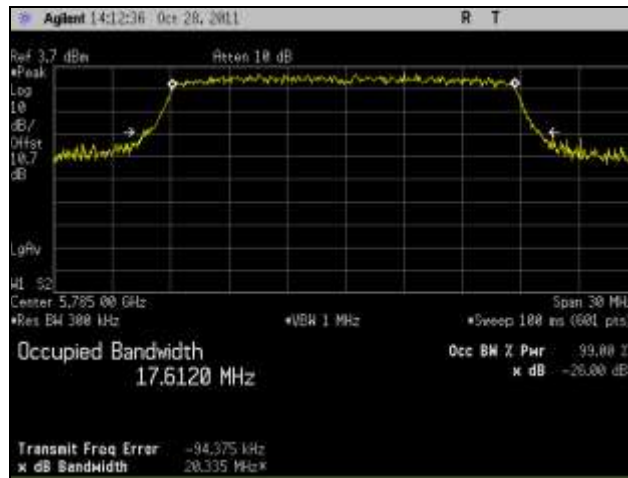
Plot 30. 26 dB Occupied Bandwidth, Mid Channel, 802.11n 20 MHz, Port 1
