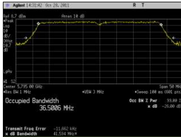
Plot 43. 26 dB Occupied Bandwidth, High Channel, 802.11n 40 MHz, Port 3
