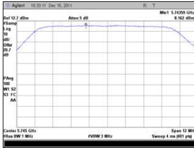
Plot 128. Power Spectral Density, Low Channel, 802.11n 10 MHz, Port 1
