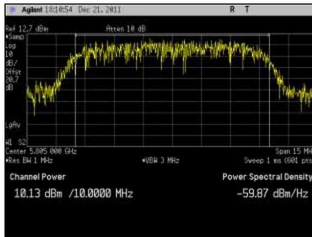
Plot 94. RF Power Output, High Channel, 802.11n 10 MHz Port 1
