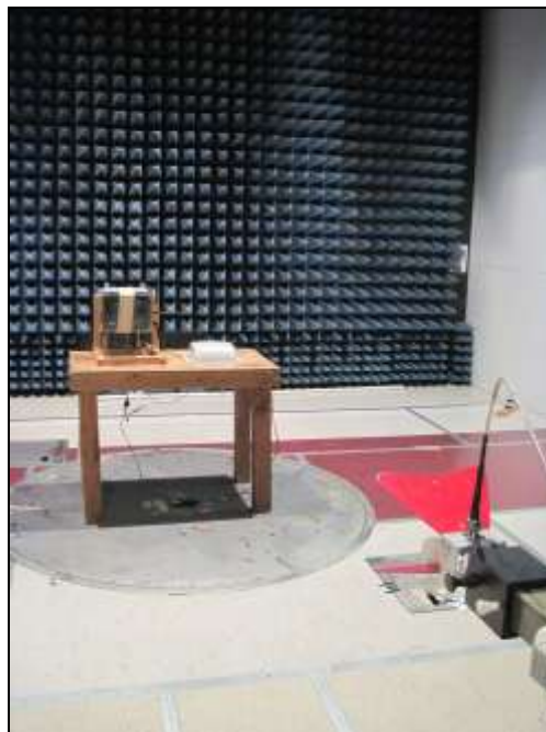
Photograph 4. Radiated Emission, 1GHz – 2GHz, Test Setup
