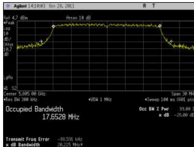
Plot 34. 26 dB Occupied Bandwidth, High Channel, 802.11n 20 MHz, Port 2
