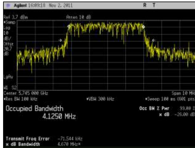
Plot 47. 99% Occupied Bandwidth, Low Channel, 802.11n 5 MHz, Port 1
