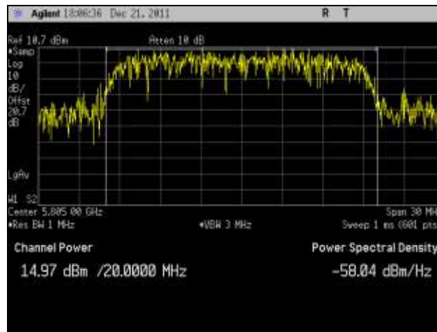
Plot 106. RF Power Output, High Channel, 802.11n 20 MHz Port 2
