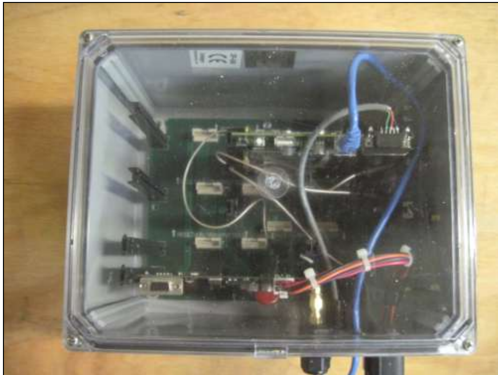
Photograph 1. Firetide, Inc. FT 5900 Wireless Mesh Node
