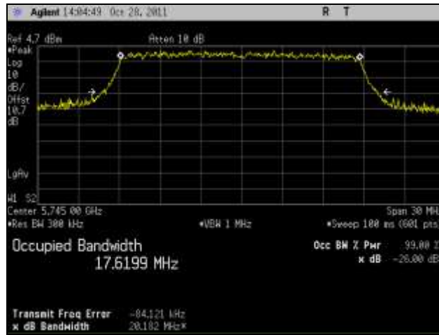
Plot 35. 26 dB Occupied Bandwidth, Low Channel, 802.11n 20 MHz, Port 3
