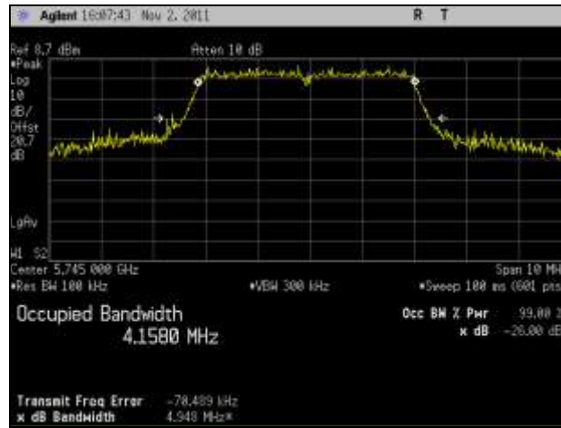
Plot 17. 26 dB Occupied Bandwidth, Low Channel, 802.11n 5 MHz, Port 3
