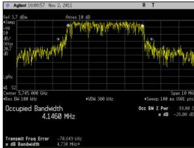
Plot 50. 99% Occupied Bandwidth, Low Channel, 802.11n 5 MHz, Port 2
