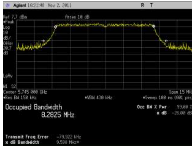
Plot 20. 26 dB Occupied Bandwidth, Low Channel, 802.11n 10 MHz, Port 1
