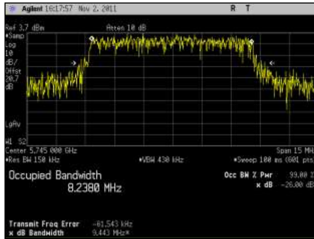
Plot 59. 99% Occupied Bandwidth, Low Channel, 802.11n 10 MHz, Port 2
