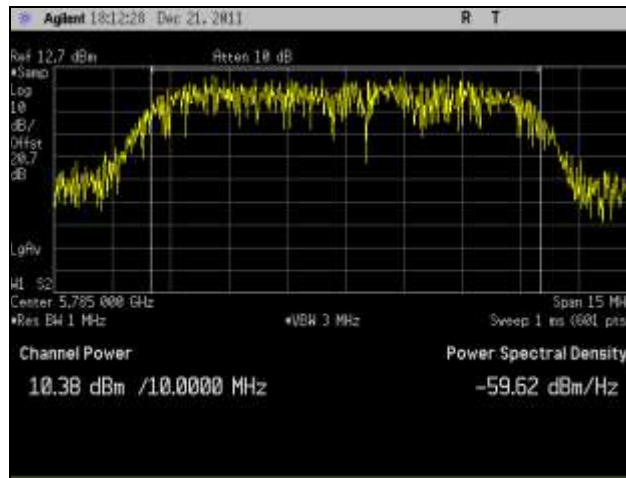
Plot 99. RF Power Output, Mid Channel, 802.11n 10 MHz Port 3
