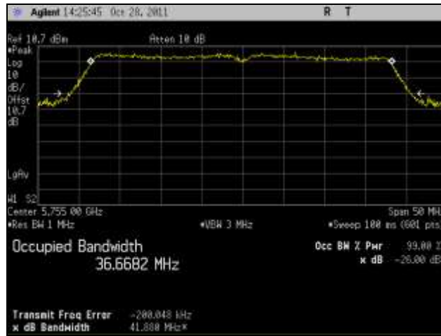
Plot 40. 26 dB Occupied Bandwidth, Low Channel, 802.11n 40 MHz, Port 2
