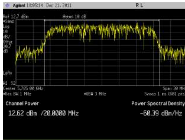
Plot 102. RF Power Output, Mid Channel, 802.11n 20 MHz Port 1
