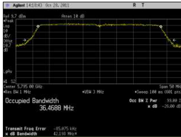
Plot 39. 26 dB Occupied Bandwidth, High Channel, 802.11n 40 MHz, Port 1
