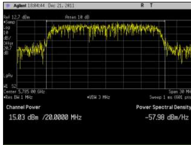
Plot 105. RF Power Output, Mid Channel, 802.11n 20 MHz Port 2
