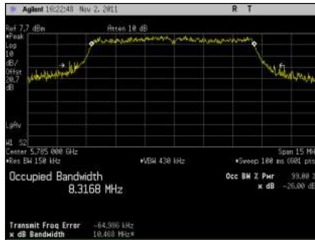
Plot 24. 26 dB Occupied Bandwidth, Mid Channel, 802.11n 10 MHz, Port 2
