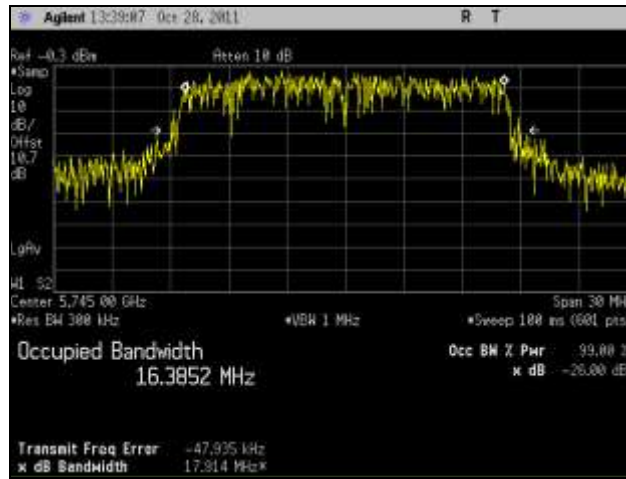
Plot 44. 99% Occupied Bandwidth, Low Channel, 802.11a
