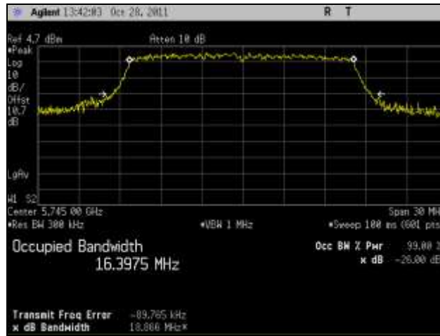
Plot 8. 26 dB Occupied Bandwidth, Low Channel, 802.11a
