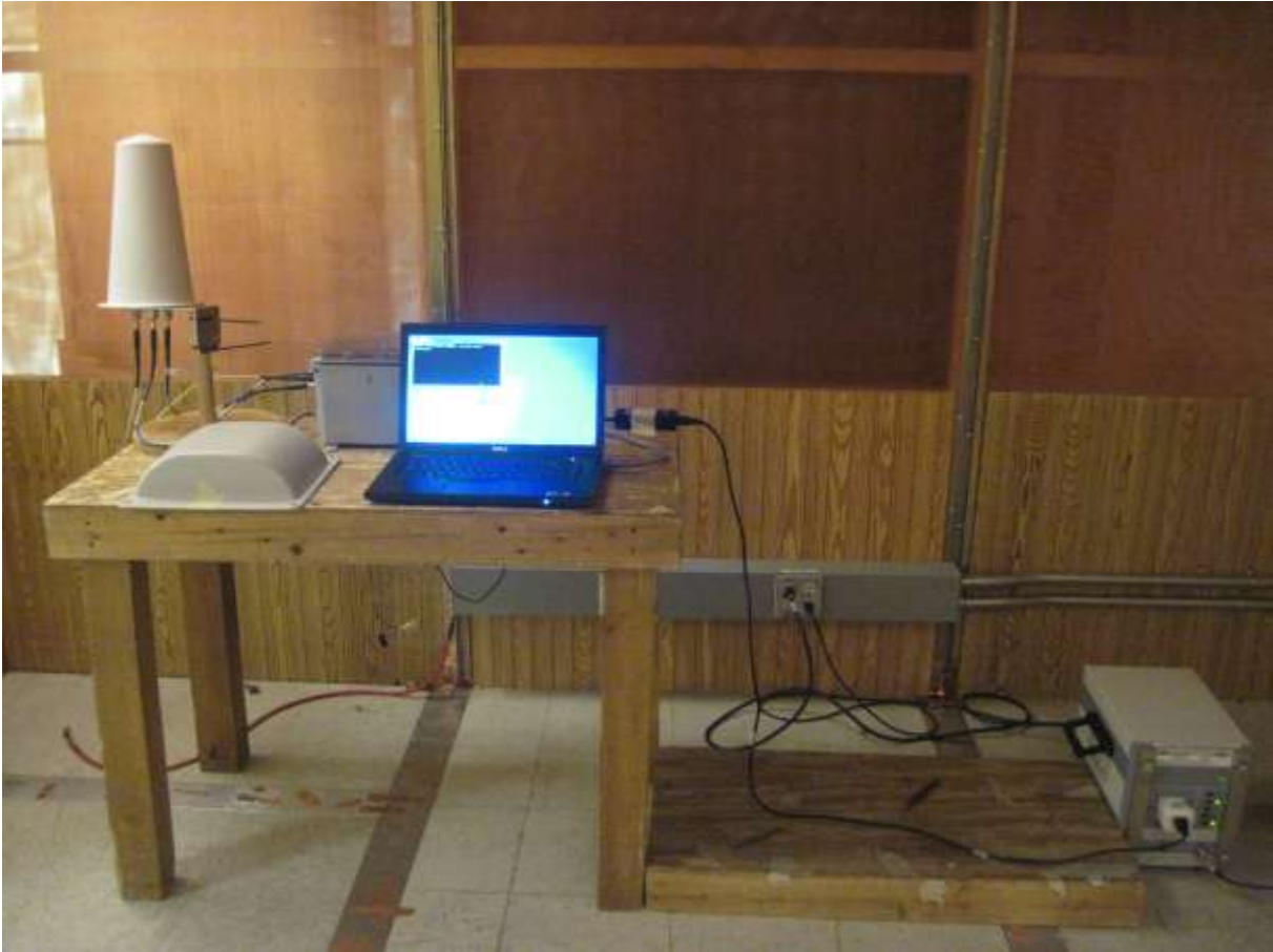
Photograph 5. Conducted Emissions, 15.207(a), Test Setup
