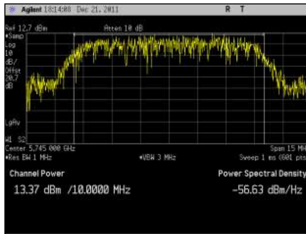
Plot 95. RF Power Output, Low Channel, 802.11n 10 MHz Port 2
