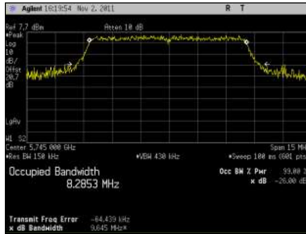
Plot 23. 26 dB Occupied Bandwidth, Low Channel, 802.11n 10 MHz, Port 2
