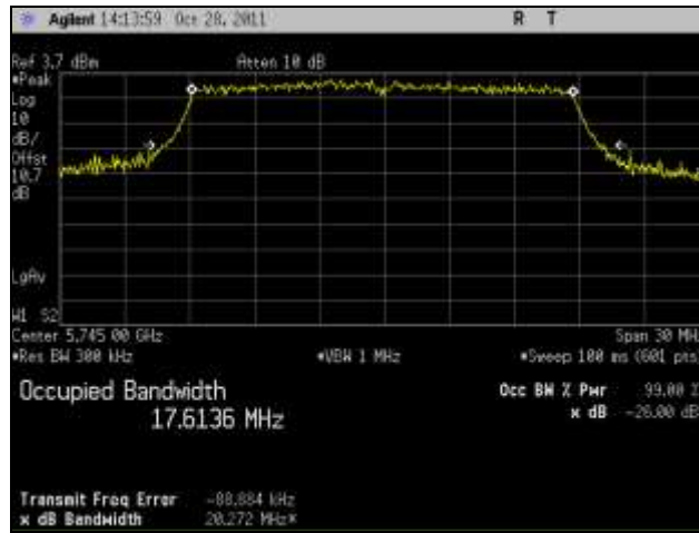
Plot 29. 26 dB Occupied Bandwidth, Low Channel, 802.11n 20 MHz, Port 1
