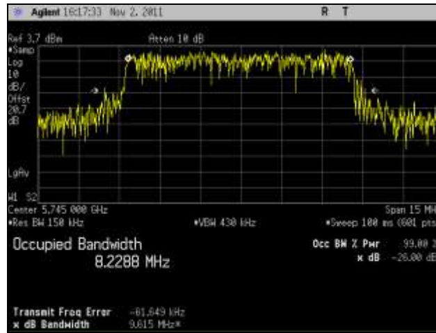
Plot 56. 99% Occupied Bandwidth, Low Channel, 802.11n 10 MHz, Port 1
