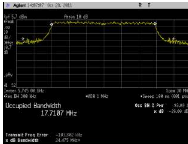
Plot 32. 26 dB Occupied Bandwidth, Low Channel, 802.11n 20 MHz, Port 2
