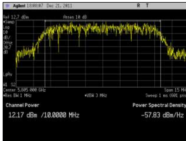
Plot 100. RF Power Output, High Channel, 802.11n 10 MHz Port 3
