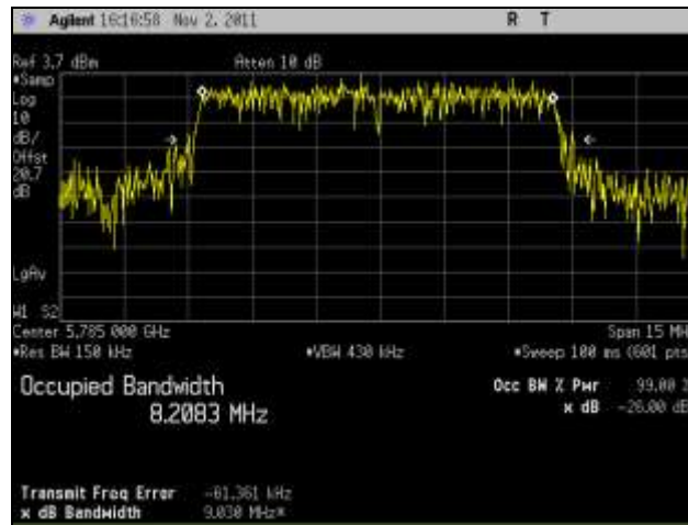
Plot 57. 99% Occupied Bandwidth, Mid Channel, 802.11n 10 MHz, Port 1
