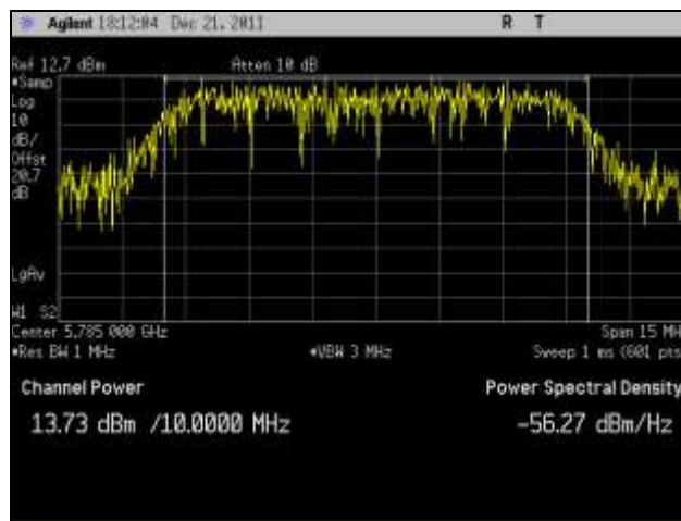
Plot 96. RF Power Output, Mid Channel, 802.11n 10 MHz Port 2
