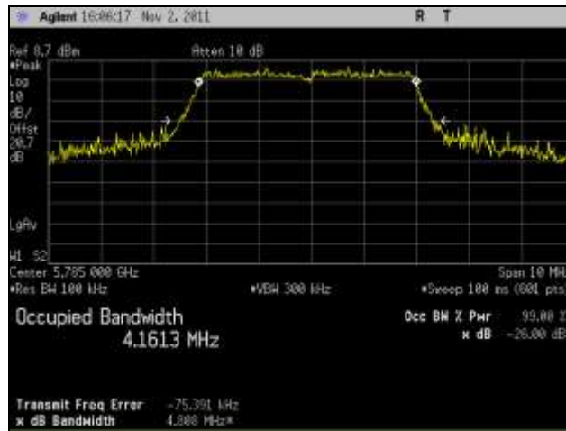
Plot 12. 26 dB Occupied Bandwidth, Mid Channel, 802.11n 5 MHz, Port 1
