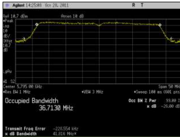
Plot 41. 26 dB Occupied Bandwidth, High Channel, 802.11n 40 MHz, Port 2
