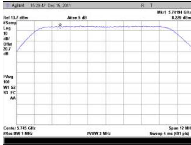
Plot 134. Power Spectral Density, Low Channel, 802.11n 10 MHz, Port 3
