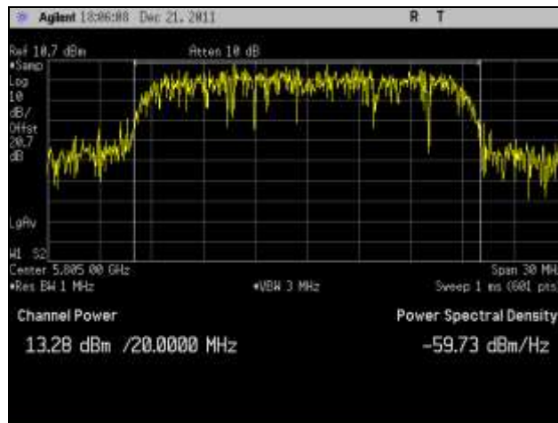
Plot 103. RF Power Output, High Channel, 802.11n 20 MHz Port 1
