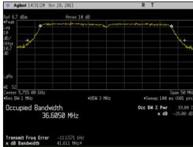
Plot 42. 26 dB Occupied Bandwidth, Low Channel, 802.11n 40 MHz, Port 3
