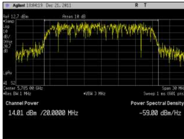
Plot 108. RF Power Output, Mid Channel, 802.11n 20 MHz Port 3
