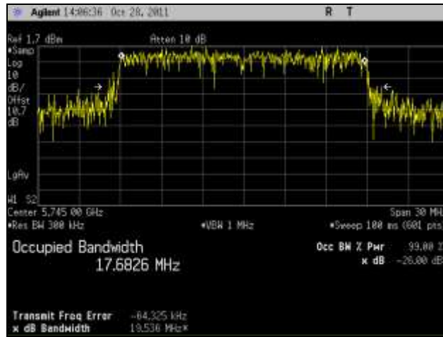
Plot 68. 99% Occupied Bandwidth, Low Channel, 802.11n 20 MHz, Port 2
