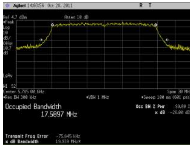
Plot 36. 26 dB Occupied Bandwidth, Mid Channel, 802.11n 20 MHz, Port 3
