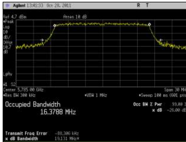
Plot 9. 26 dB Occupied Bandwidth, Mid Channel, 802.11a
