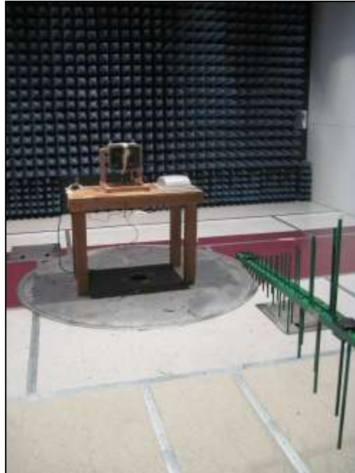
Photograph 3. Radiated Emission, 30MHz – 1GHz, Test Setup
