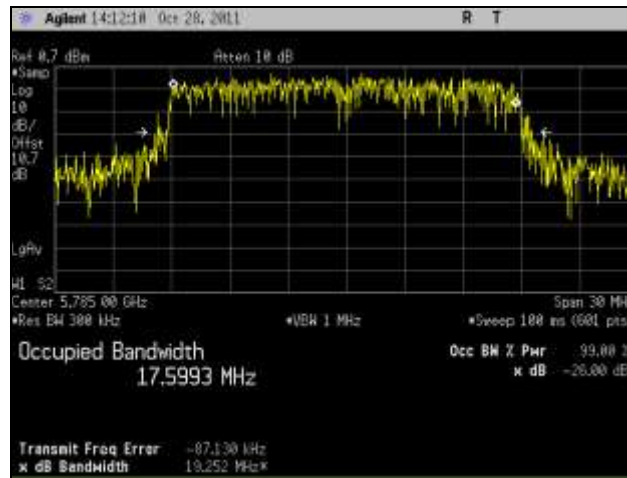
Plot 66. 99% Occupied Bandwidth, Mid Channel, 802.11n 20 MHz, Port 1
