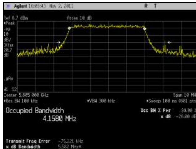
Plot 19. 26 dB Occupied Bandwidth, High Channel, 802.11n 5 MHz, Port 3
