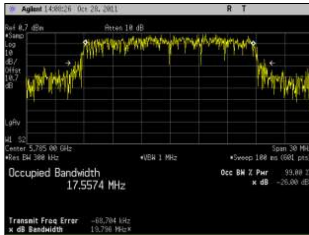
Plot 69. 99% Occupied Bandwidth, Mid Channel, 802.11n 20 MHz, Port 2
