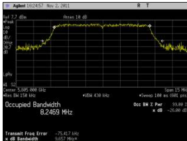
Plot 22. 26 dB Occupied Bandwidth, High Channel, 802.11n 10 MHz, Port 1
