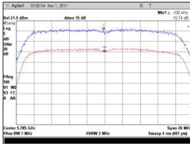
Plot 174. Peak Excursion Ratio, Mid Channel, 802.11n 20 MHz, Port 1
