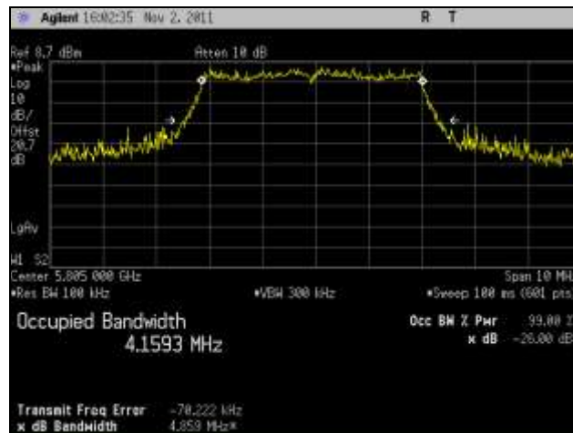
Plot 16. 26 dB Occupied Bandwidth, High Channel, 802.11n 5 MHz, Port 2
