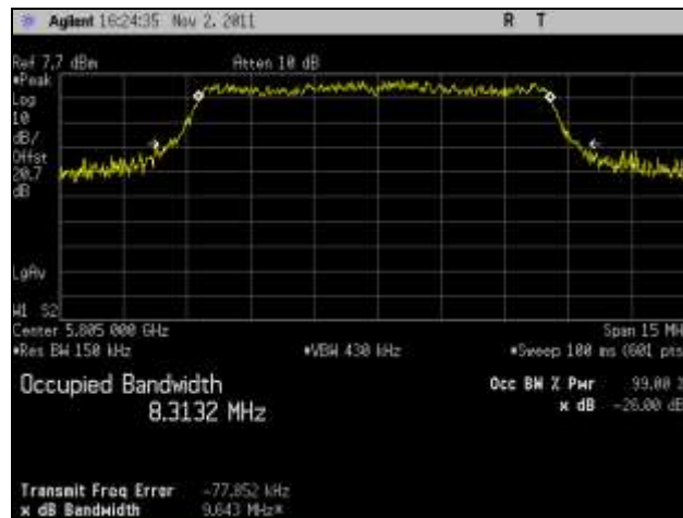
Plot 25. 26 dB Occupied Bandwidth, High Channel, 802.11n 10 MHz, Port 2
