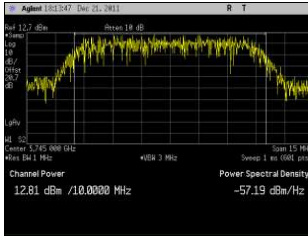
Plot 98. RF Power Output, Low Channel, 802.11n 10 MHz Port 3
