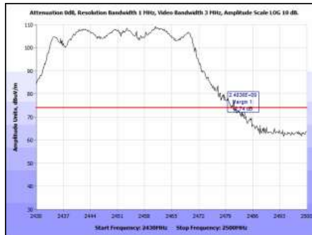
Plot 578. Radiated Restricted Band Edge, High Channel (2452 MHz), Peak, 802.11n 40 MHz, 5 dBi Omni, 2.4 GHz
