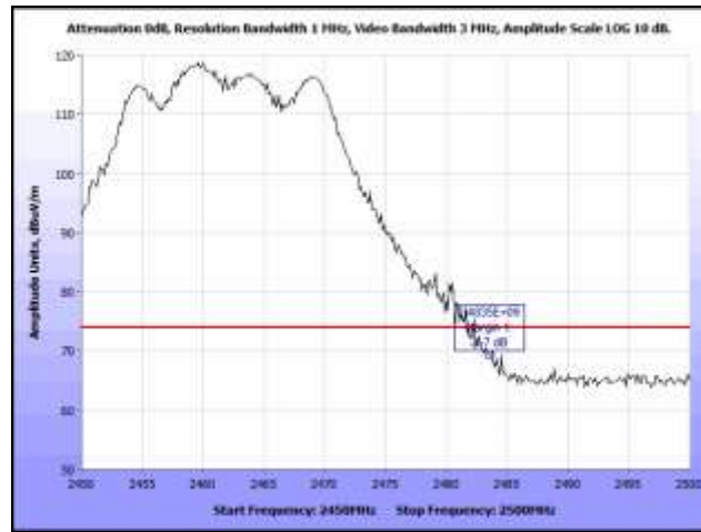
Plot 564. Radiated Restricted Band Edge, High Channel (2462 MHz), Peak, 80.21n 20 MHz, 5 dBi Omni, 2.4 GHz
