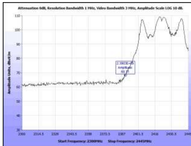
Plot 604. Radiated Restricted Band Edge, Low Channel, Peak, 802.11n 40 MHz, 8 dBi Omni, 2.4 GHz
