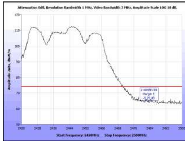
Plot 574. Radiated Restricted Band Edge, High Channel (2442 MHz), Peak, 802.11n 40 MHz, 5 dBi Omni, 2.4 GHz
