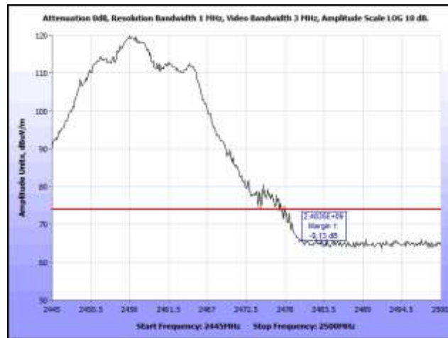
Plot 562. Radiated Restricted Band Edge, High Channel (2457 MHz), Peak, 802.11n 20 MHz, 5 dBi Omni, 2.4 GHz
