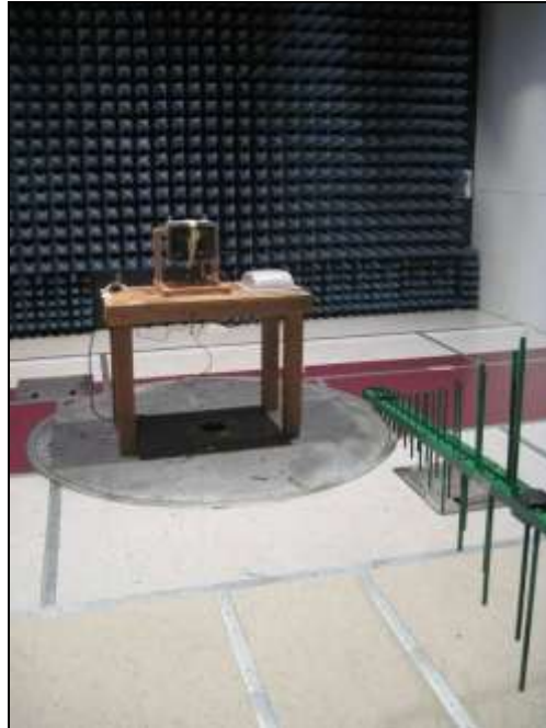
Photograph 3. Radiated Emission, 30MHz – 1GHz, Test Setup
