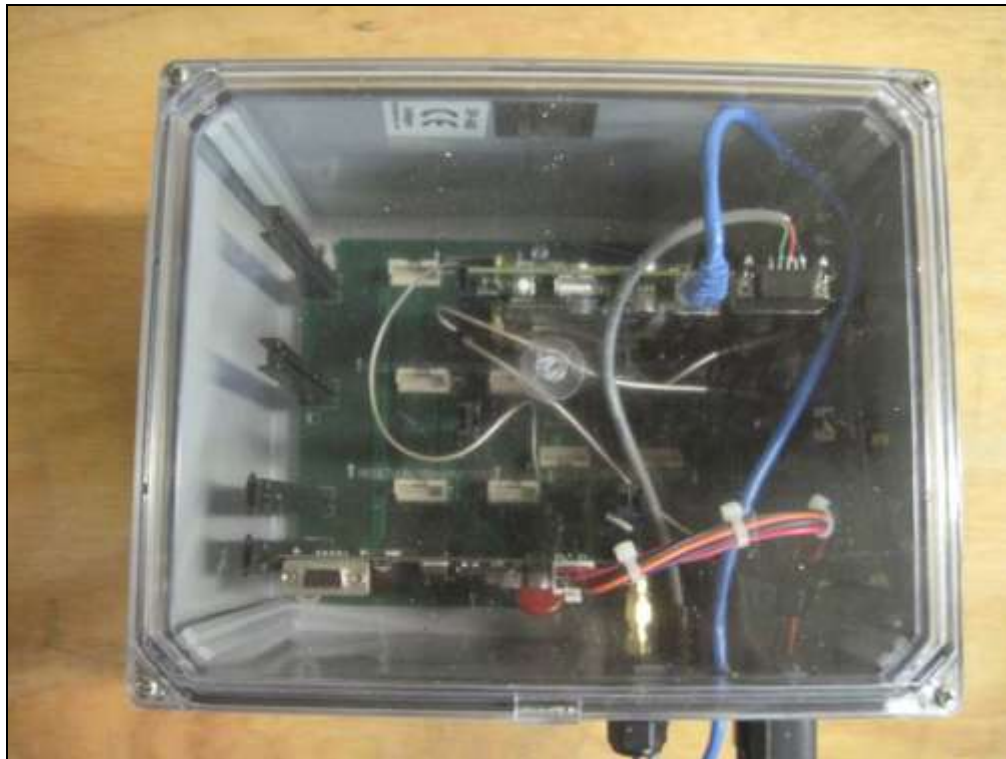
Photograph 1. Firetide, Inc. FT 5900 Wireless Mesh Node
