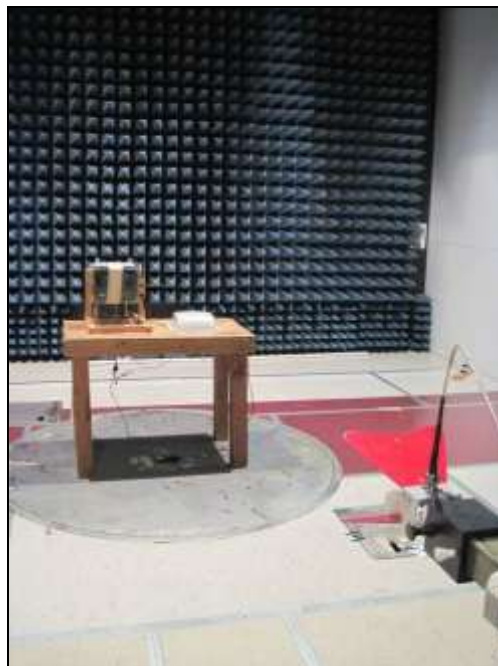
Photograph 4. Radiated Emission, 1GHz – 2GHz, Test Setup
