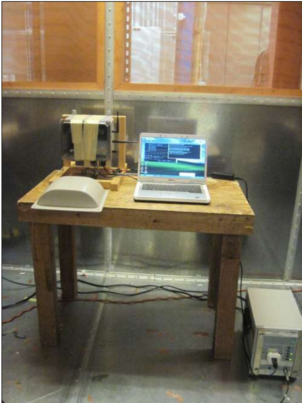
Photograph 5. Conducted Emissions, 15.207(a), Test Setup, 2.4 GHz
