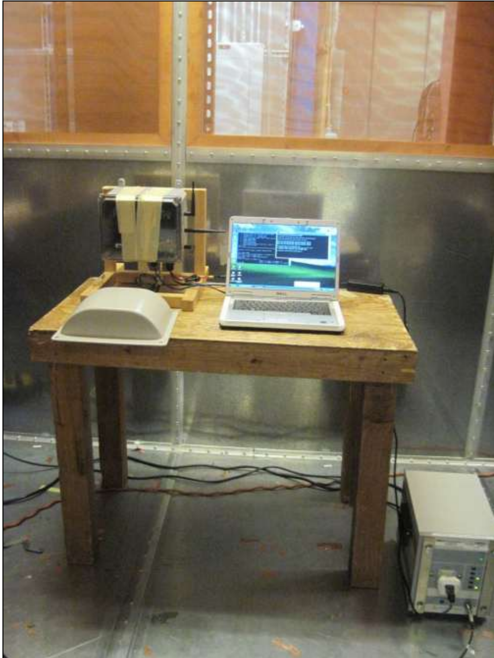
Photograph 2. Conducted Emissions, Test Setup
