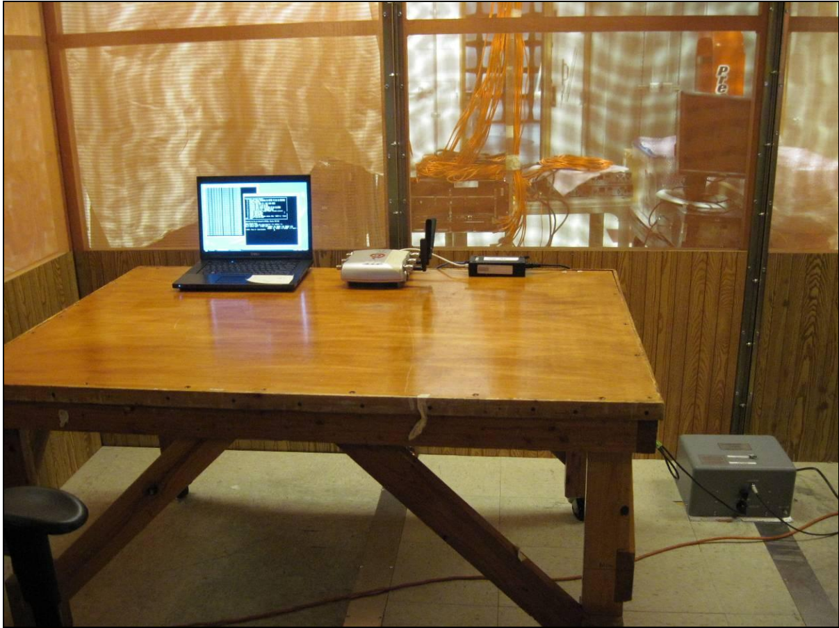
Photograph 5. Conducted Emissions (15.207) Test Setup PoE30U-560
