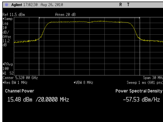
Plot 82. RF Power Output, 802.11a, 5320 MHz
