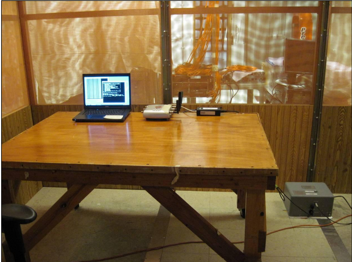
Photograph 3. Conducted Emissions, Test Setup PoE30U-560
